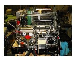
Components – Fuel Cell Stack and Heat Exchanger
