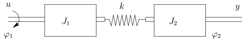
$$\begin{aligned} J_1 \ddot{\varphi}_1 &= u - \tau_1 & y &= \dot{\varphi}_2 + f \\ \tau_1 &= k(\varphi_1 - \varphi_2) \\ J_2 \ddot{\varphi}_2 &= \tau_1 \end{aligned}$$
