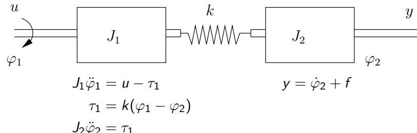
$$\begin{aligned} J_1 \ddot{\varphi}_1 &= u - \tau_1 & y &= \dot{\varphi}_2 + f \\ \tau_1 &= k(\varphi_1 - \varphi_2) \\ J_2 \ddot{\varphi}_2 &= \tau_1 \end{aligned}$$
