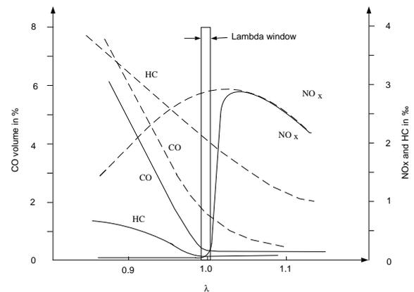
**Figure 1. Dashed: Emissions before the catalyst. Solid: Emissions after the catalyst. When  $\lambda$  is close to unity the three way catalyst (TWC) effectively removes the three pollutants CO, HC, and  $NO_x$ .**
