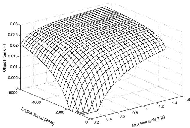
**Figure 8. Result using an I-controller with delayed switching. The figure shows the maximum mean deviation from stoichiometric with these settings.**
