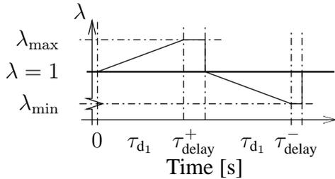
**Figure 6. Delayed switching with time  $\tau_{\text{delay}}^+$  during lean conditions and  $\tau_{\text{delay}}^-$  during rich conditions.**
