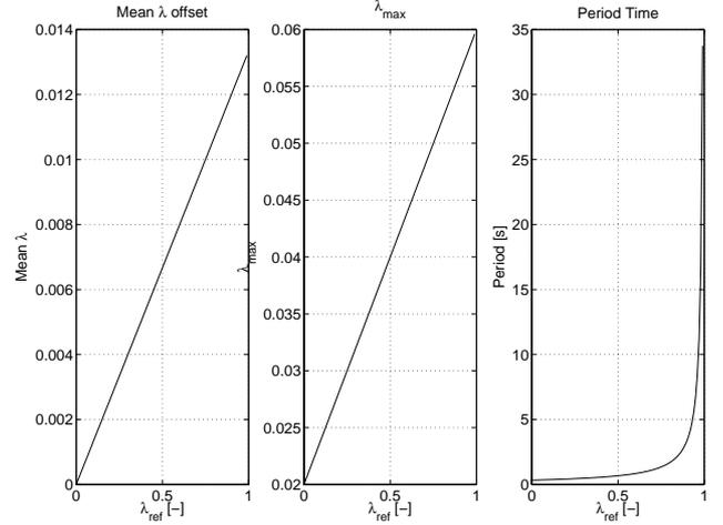
**Figure 7. Result using the straight forward approach with varying  $\lambda_{ref}$  using  $\tau_{d_1} = 110$  ms, and  $A = 0.02$ . To the left the maximum obtainable  $\bar{\lambda}$  is shown and in the middle  $\lambda_{max}$  is shown. The maximum amplitude exceeds the desired amplitude of 0.02 for  $\lambda_{ref} > 0$ . To the right the period time  $T$  is shown which is small for  $\lambda_{ref} < 0.8$ .**
