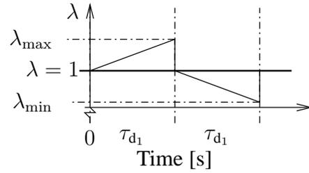
**Figure 5.  $\lambda_{\text{engine}}$ -output with PI-control and  $K_p$  and  $K_I$  calculated as described in Equations (10,11).  $\lambda_{\text{max}} = A = -\lambda_{\text{min}}$ . The time delay until the mixture reaches the sensor is  $\tau_{d_1}$ .**
