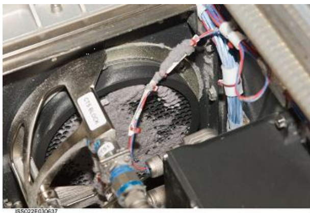
FIGURE 6. Dust Collection in the air loop
