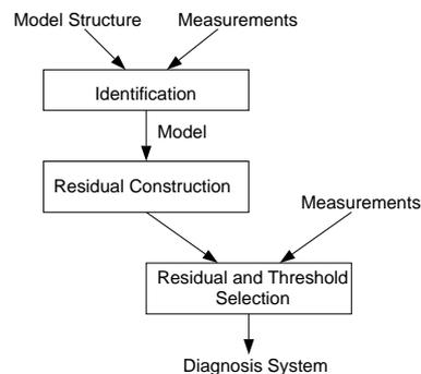
Fig. 1. The process of constructing a FDI system.
