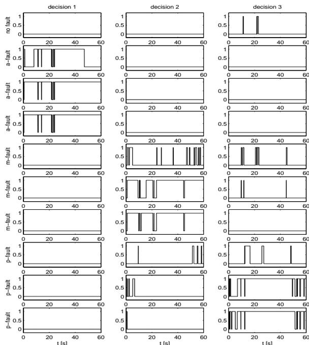
Fig. 5. Confirmation of the FDI design for the cases no fault,  $\alpha$ -,  $m$ -, and  $p$ -fault respectively.
