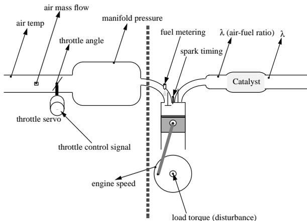
Fig. 2. The basic SI-engine.
