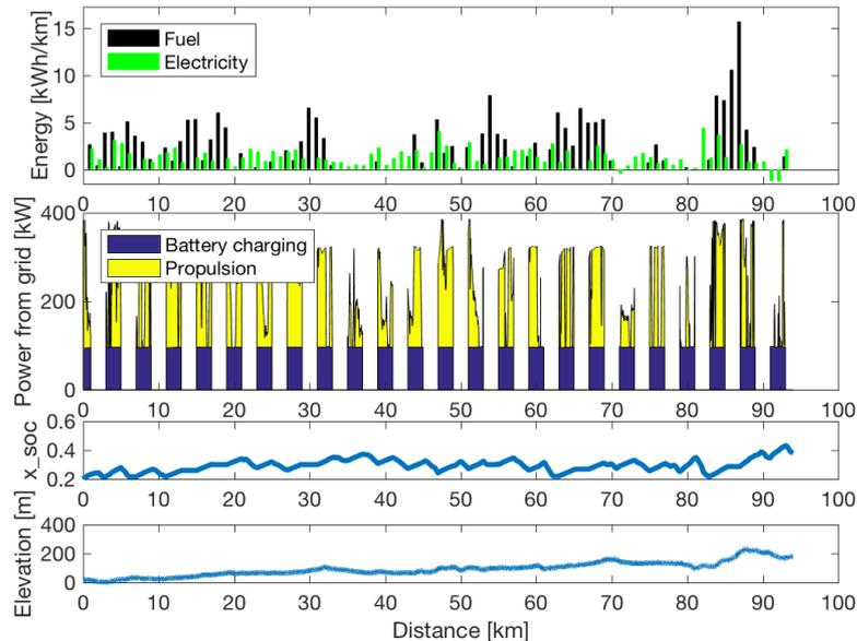
Fig. 7. Case 3: Half distance electrified in sequences of 2 km. No maximum power limit from the grid.
