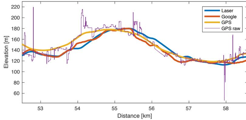
Fig. 4. Elevation data from three different sources. Both the raw GPS data and filtered data are presented
