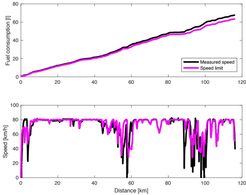
Figure 3: The upper plot presents the fuel consumption when the reference speed in the simulations are based on measurement speed data and speed limit data. The simulated speed profiles are presented in the lower plot for corresponding reference speed profiles. The simulated average speed is 67 km/h when the measured speed data is used and 74km/h when the speed limit data is used. The simulated road is Gävle-Borlänge and a conventional vehicle with only an engine is considered.
