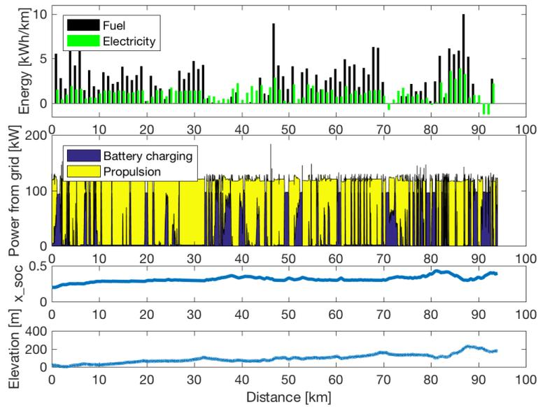
Fig. 6. Case 2: All distance electrified, but the maximum power from the grid is 130 kW.
