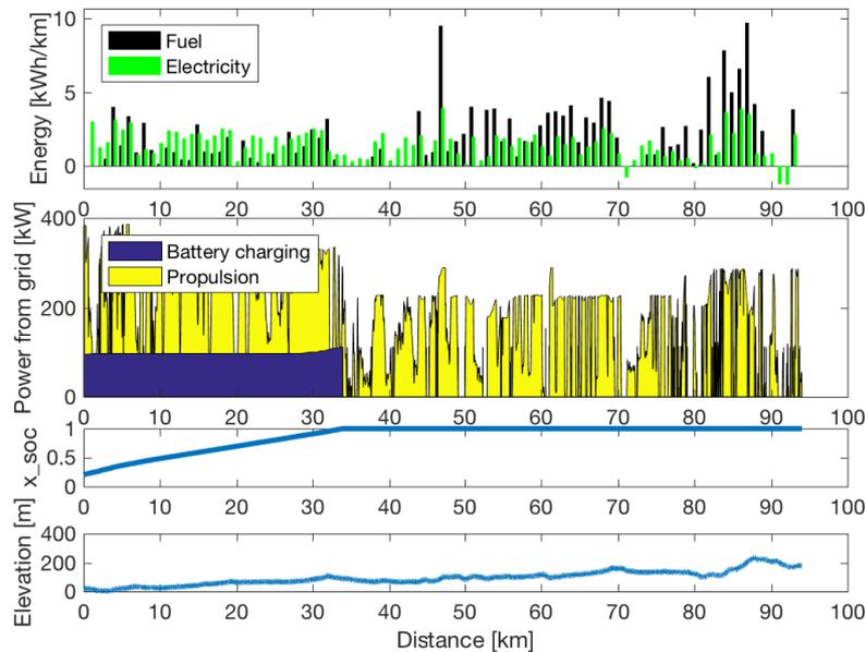
Fig. 5. Case 1: The electric grid is available with no power limits at the entire road.
