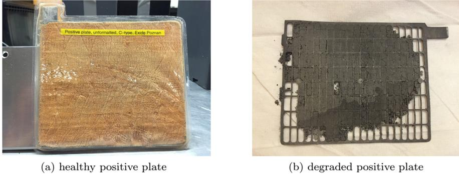
Figure 1.2: Healthy, left figure, and degraded, right figure, positive plates in lead acid batteries.
