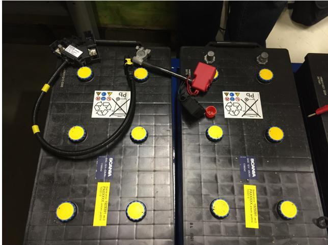
Figure 1.1: Lead-acid starter battery used at Scania CV.
