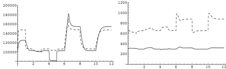
Figure 8.3: Modelica MVEM driving a load. Left: pressures [Pa] in inlet (solid) and exhaust (dashed) manifolds. Right: temperatures [K] in manifolds.
