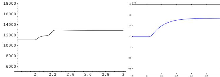
Figure 8.13: Step in turbine vanes, turbo speed [rad/s]. Left: Modelica, right: Simulink.
