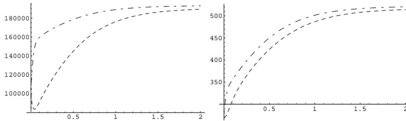
Figure 7.5: Simulation of Closed system. Left: pressures [Pa] in the low (dashed) and high (dot-dashed) volumes. Right: temperatures [K] in the volumes.
