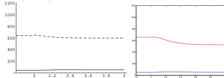
Figure 8.16: Step in turbine vanes, temperatures [°C] in inlet (solid) and exhaust (dashed) manifolds. Left: Modelica, right: Simulink.
