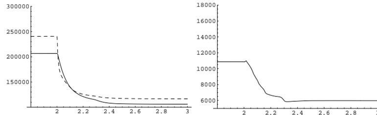
Figure 8.7: Modelica MVEM back-flow. Left: pressures [Pa] in inlet (solid) and exhaust (dashed) manifolds. Right: turbo speed [rad/s].
