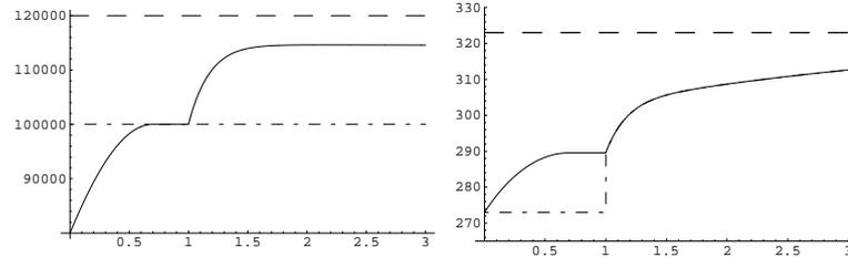
Figure 7.2: Simulation of Simple system. Left: pressures [Pa] in *Volume* (solid) and reservoirs (dashed and dot-dashed). Right: temperatures [K] in *Volume* (solid), *Valve* (dashed) and *Restriction* (dot-dashed). Time [s] on x-axes.
