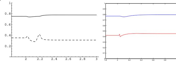
Figure 8.14: Step in turbine vanes, compressor (solid) and turbine (dashed) efficiencies. Left: Modelica, right: Simulink.
