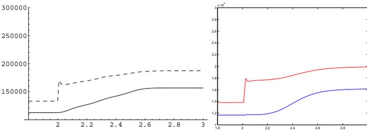
Figure 8.11: Step in fuel-injection, pressure [Pa] in inlet (solid) and exhaust (dashed) manifolds. Left: Modelica, right: Simulink.
