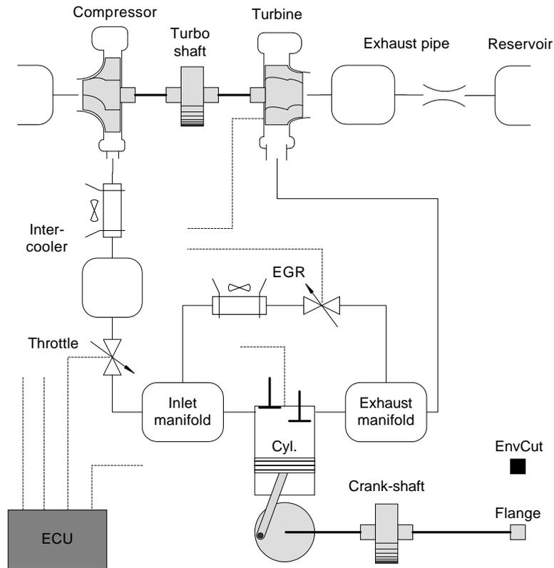
Figure 8.1: Topology of Modelica OM611 MVEM. Thermodynamic connections in solid, mechanical in thick solid and signal in dashed lines.
