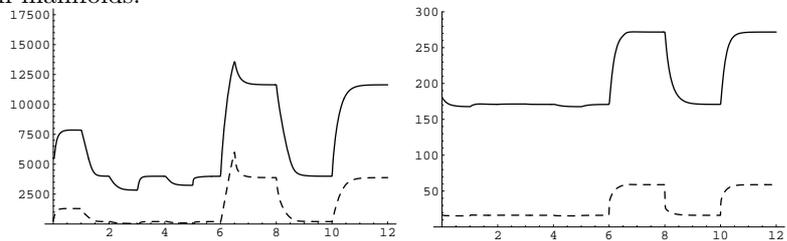
Figure 8.4: Modelica MVEM driving a load, speeds (solid) and powers (dashed). Left: turbo speed [rad/s] and power [W]. Right: engine speed [rad/s] and power [kW].
