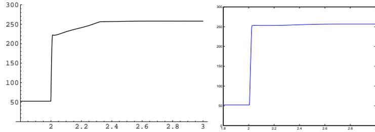
Figure 8.9: Step in fuel-injection, engine torque [Nm]. Left: Modelica, right: Simulink.
