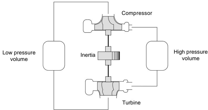
Figure 7.4: Closed system with turbo.
