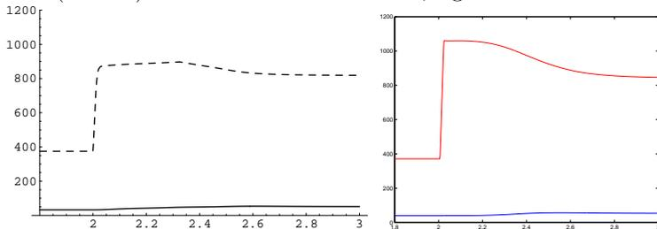
Figure 8.12: Step in fuel-injection, temperatures [°C] in inlet (solid) and exhaust (dashed) manifolds. Left: Modelica, right: Simulink.
