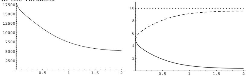
Figure 7.6: Simulation of Closed system. Left: turbo-speed [rad/s]. Right: kinetic (solid), thermal (dashed) and total (dotted) energies [kJ].
