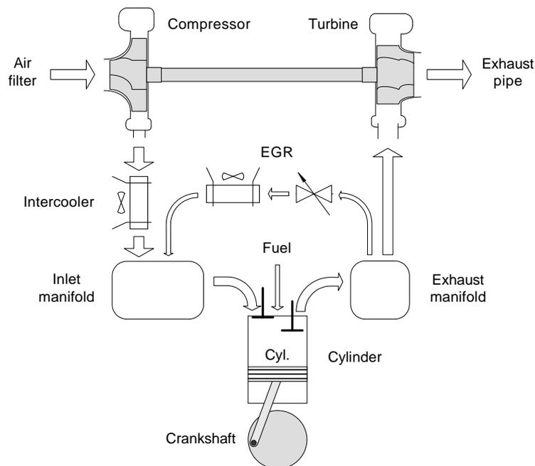
Figure 2.1: Gas path through a typical modern diesel engine.
