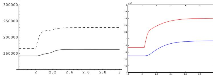
Figure 8.15: Step in turbine vanes, pressure [Pa] in inlet (solid) and exhaust (dashed) manifolds. Left: Modelica, right: Simulink.
