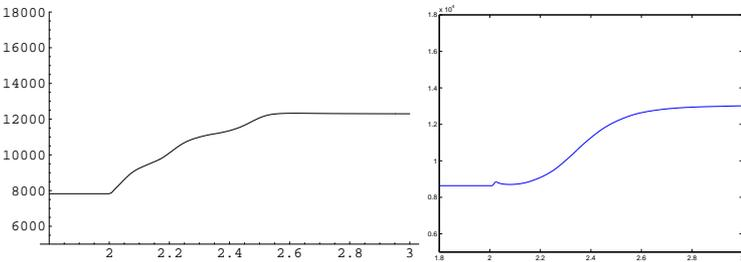
Figure 8.10: Step in fuel-injection, turbo speed [rad/s]. Left: Modelica, right: Simulink.
