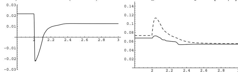
Figure 8.8: Modelica MVEM back-flow. Left: mass-flow [kg/s] through EGR-valve. Right: mass-flows [kg/s] through compressor (solid) and turbine (dashed).
