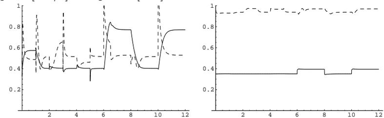
Figure 8.5: Modelica MVEM driving a load. Left: compressor (solid) and turbine (dashed) efficiencies. Right: combustion (solid) and volumetric (dashed) efficiencies.
