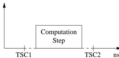
Figure 4.1: To measure the computation time for a given step in a model, the time  $TSC2 - TSC1$  is calculated and stored into a file. The measured time may be extended by interrupt latencies both before and after the computation step of the model.
