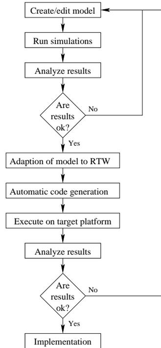
Figure 2.1: Rapid prototyping development process.
