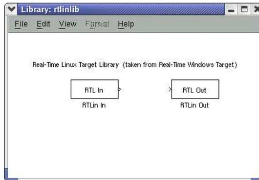
Figure 3.10: The *rtlinlib* block library containing the device driver blocks *RTL In* and *RTL Out*.
