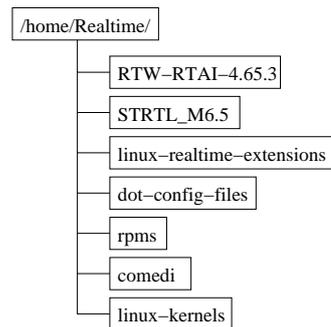
Figure 3.2: The directory structure of the software packages and configuration files.
