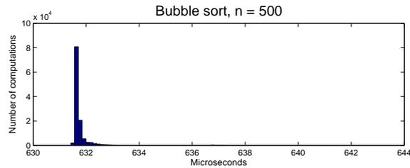
Figure 4.6: Histogram showing the variation of computation times needed for the algorithm bubble sort; where  $n = 500$ , sample time = 0.001 seconds, and the duration of the test =  $\sim 2$  minutes.
