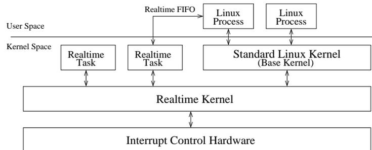
Figure 2.3: Flow of data and control. Ordinary Linux processes execute in user space, a protected environment, while the Linux kernel and the realtime tasks execute in kernel space, without protection against programming errors. Linux processes and realtime tasks communicate, e.g., via realtime FIFOs.
