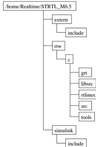
Figure 3.5: The directory structure of STRTL\_M6.5. The directory `extern/include` contains header and `.mlib` files. Under the `rtw/c` directory the important directories are `rtlinux` and `src`. The directory `simulink/include` contains Matlab header files.
