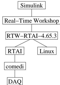
Figure 3.7: System overview with RTAI as the hard realtime execution component and RTW-RTAI-4.65.3 as the component conforming the automatically Real-Time Workshop generated code to be runnable on RTAI.
