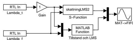
Figure 4.8: A linear adaptive model of a catalyst system.
