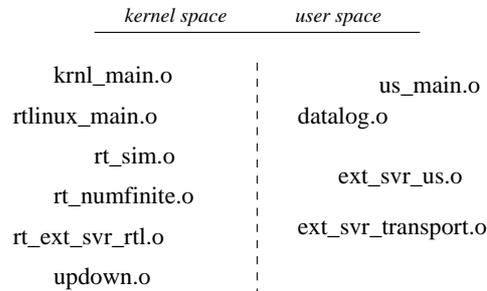
Figure 3.6: The modules are separated into kernel space and user space. The communication between modules is achieved by special realtime FIFOs or special realtime shared memory. The shared memory can not be swapped in and out of the hard drive.
