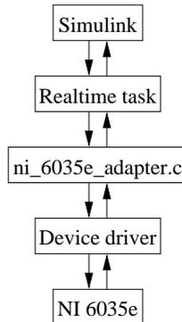
Figure 3.9: Simulink and the realtime task communicates via the external mode. The realtime task and the device driver communicates via `ni_6035e_adapter.c`, the device driver is provided by Comedi. NI 6035E is the data acquisition card.
