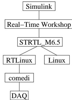
Figure 3.4: System overview with RTLinux as the hard realtime execution component and STRTL\_M6.5 as the component conforming the automatically Real-Time Workshop generated code to be runnable on RTLinux.
