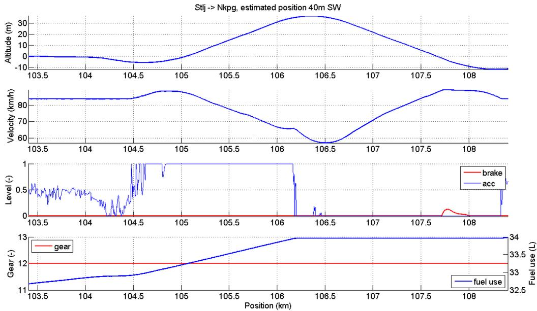
**Figure 21: Control signals, positioning error SW**
