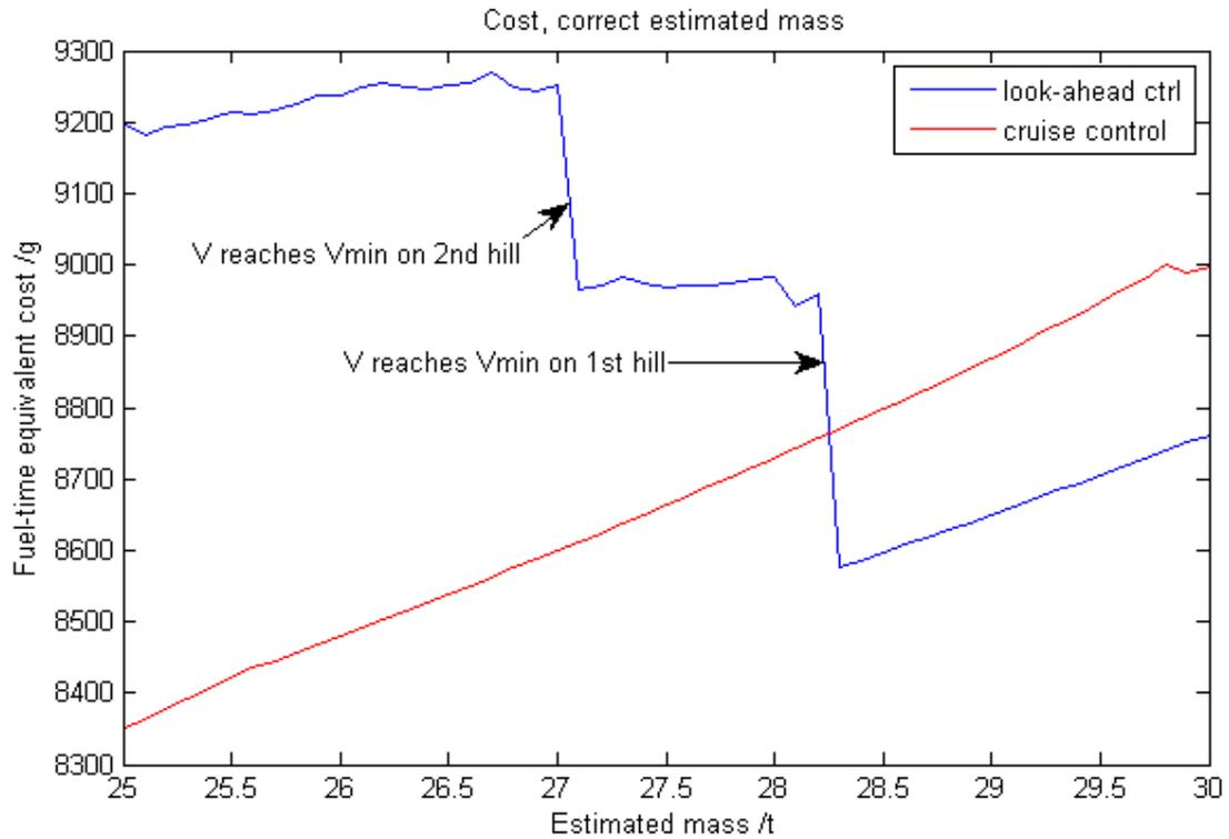
**Figure 29: Cost, correct estimated mass,  $V_{ref} = 84\text{km/h}$**
