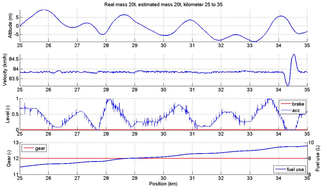
**Figure 12: Control signals, correct estimated**
