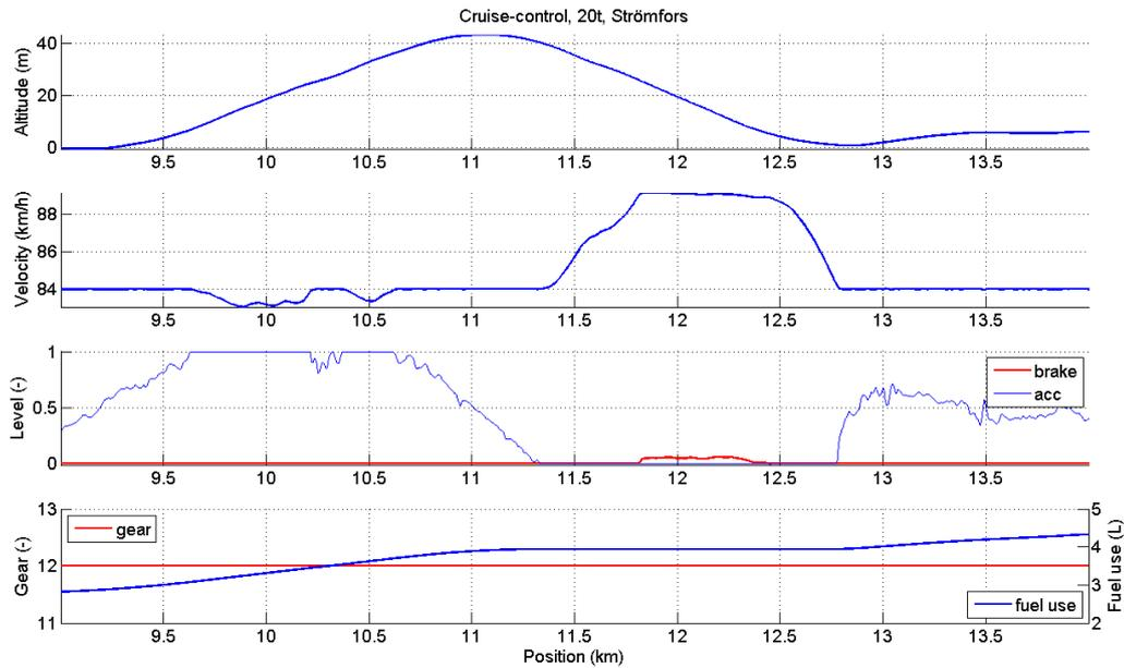
**Figure 11: Control signals, cruise control 20t**
