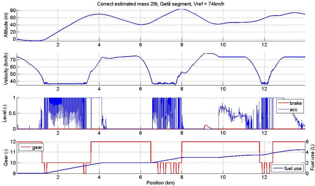
**Figure 38: Control signals, 26t,  $V_{ref} = 74\text{km/h}$**
