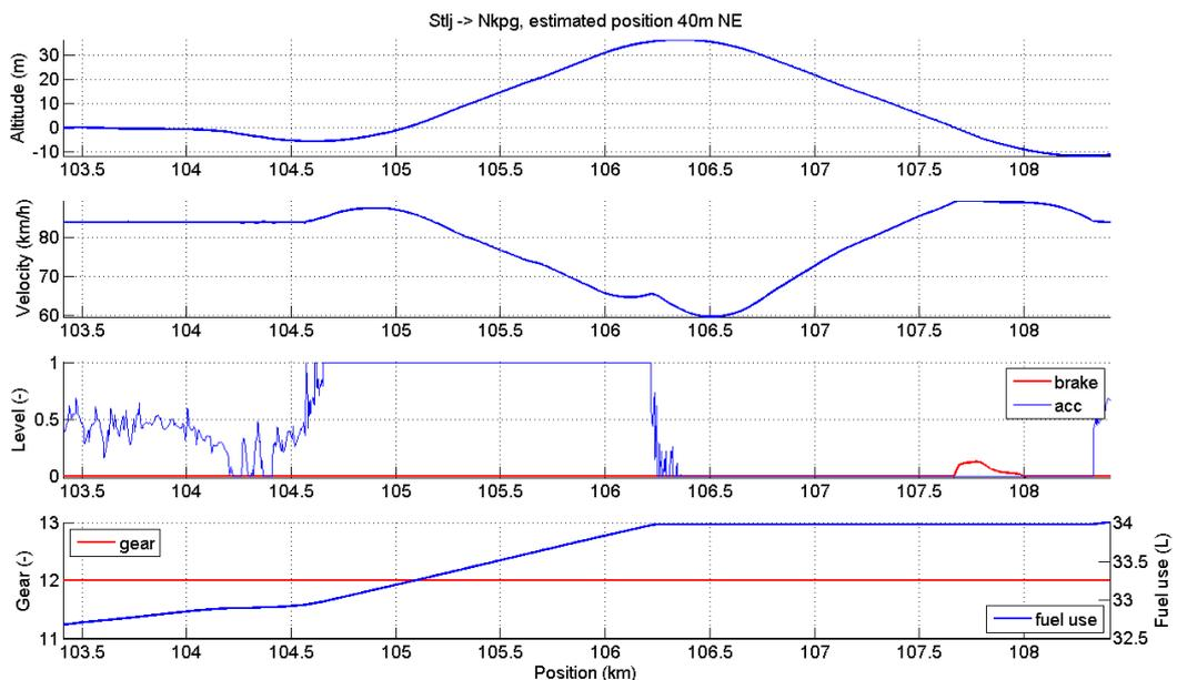
**Figure 20: Control signals, positioning error NE**
