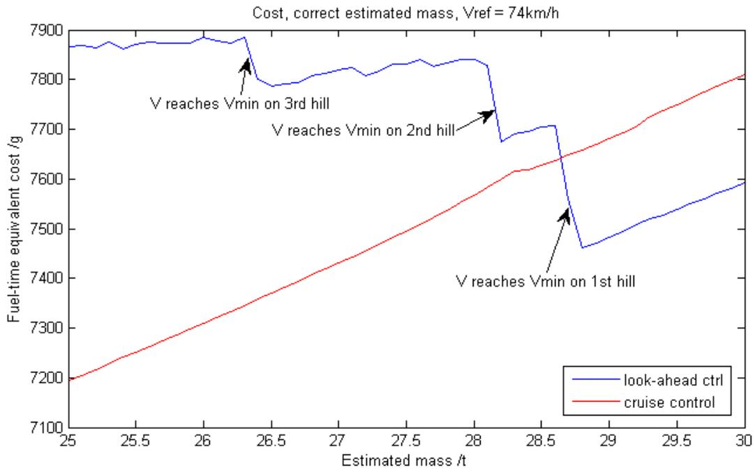
**Figure 35: Cost, correct estimated mass,  $V_{ref} = 74\text{km/h}$**
