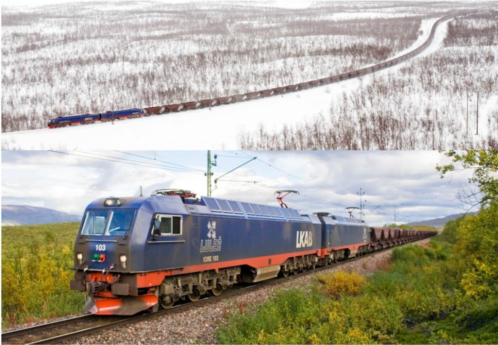
*Figure 3.5: Standard ore train configuration in north of Sweden, with two IORE locomotives followed by 52 ore wagons. (Pictures taken by David Gubler on the route Abisko – Stordalen)*
