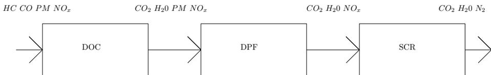
**Figure 3.2:** Aftertreatment system overview in the studied vehicle. The chemical formulas noted above the arrows defines the emissions that are present in the exhaust flow, assuming that ideal emission reduction capability is possible. After all components, the emissions are reduced to  $CO_2$ ,  $H_2O$  or  $N_2$ .
