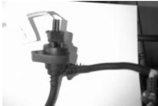
Figure 2.5: A picture of the purge control valve.
