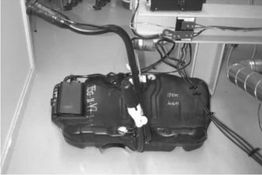
Figure 2.1: The fuel tank with the EVAP system mounted to it. The carbon canister is seen at the left of fuel tank and the diagnosis valve is the white thing next to the fuel filling-pipe.
