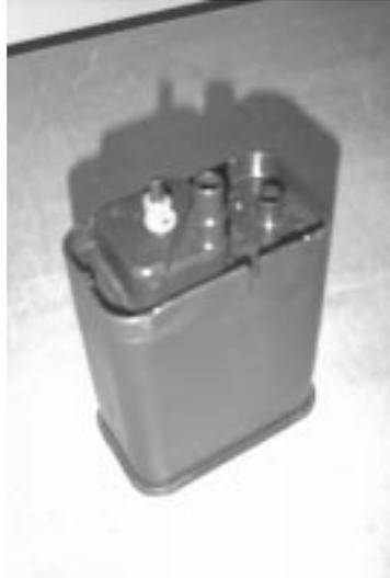
Figure 2.4: The carbon canister.
