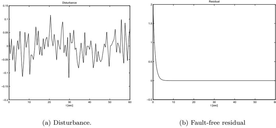
FIGURE 2. The disturbance  $d$  and the residual  $r$  in fault free simulation.
