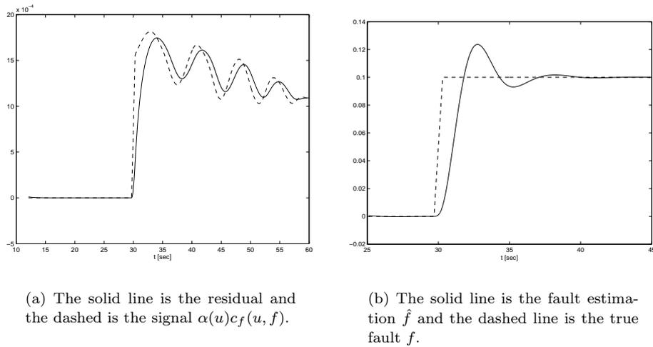
FIGURE 3. The residual and a fault estimate in the case of a 10% fault in the tangential thruster.
