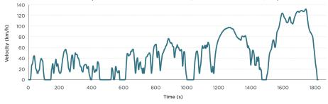
Velocity profile, WLTC (Worldwide Harmonized Light Vehicles Test Cycle)
