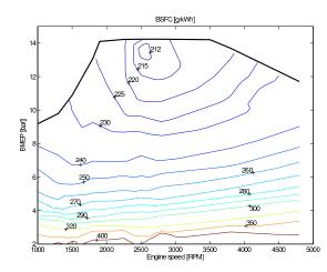
Measured engine efficiency map.
