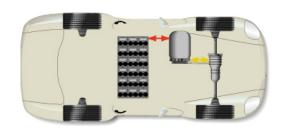
Sketch of the energy paths (Thin=Electric, Thick=Mechanic)
