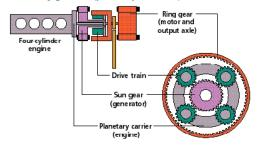
Can add more planetary gears. For example: Prius Gen 1  $\rightarrow$  Gen 2.
