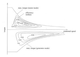
Mirroring efficiency is not always good if you need to estimate regenerative braking current
