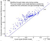
A comparison between backflow from simulations using the combustion and gas exchange model, and the cycle model. Note that only physical parameters are used, i.e. there are no fitted parameters.
