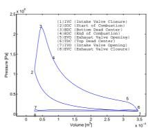
The simpler cycle model being developed focuses on the valve overlap period (point 7-8 in the figure), because this is the only period during the engine cycle when bookkeeping is really important and because the flow during this overlap is one of the larger contributors A pV-diagram showing a complete en- to the difference in the intake processes for en-
