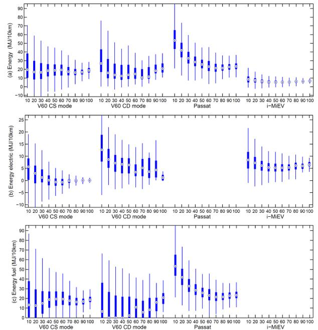
Fig. 3 Boxplots of total (top), electric (middle) and fuel (bottom) energy consumption grouped by vehicle type and vehicle speed (km/h). Outliers (outside of 2.7 standard deviations) are not shown.
