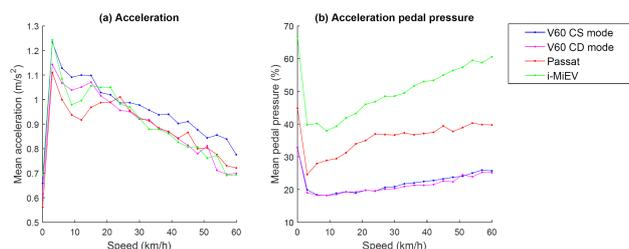
Fig. 5 The mean value, across all 5-second acceleration segments and as a function of speed, of the maximum acceleration and max accelerator pedal position within each segment.
