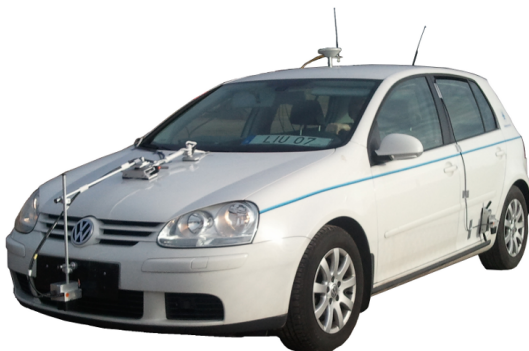
Figure 1: The LiU Research Vehicle, a vehicle testbed developed for vehicle dynamics studies.
