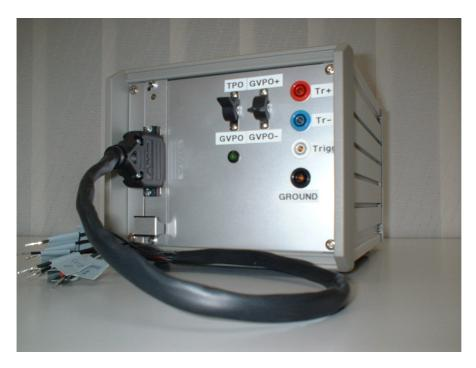
Figure 5.1. Construction of gate voltage pulsed operation. The front panel has switches to select pulse mode, temperature pulsed or gate voltage pulsed operation, and to select the sign (positive or negative potential) for the gate voltage pulsed operation mode. Temperature pulsed operation is a method to heat a sensor with controlled heat intervals. Further, the front panel has an output for trigger functions.
