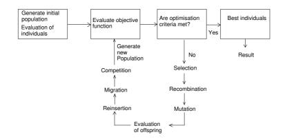
Figure 4.2: Evolutionary algorithms structure with multiple populations
