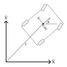
Figure 2.2: The CoG co-ordinate system in relation to the inertial.
