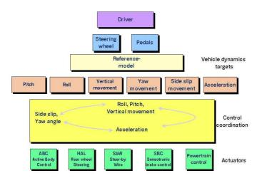
Figure 1.3: Overview of the VFD system in Technoshuttle.
