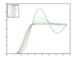
Figure 3.8: Influence of driver lead time,  $T_{L\psi}$
