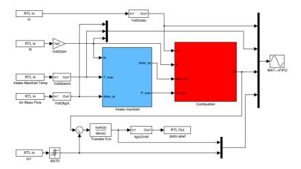
Figure 4.9: A model estimating the torque in an SVC engine and feeding a controller with the estimate.
