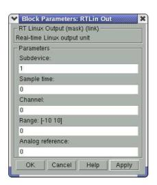
Figure 3.12: The output device driver block interface. Using the NI 6035e card: the  $Subdevice\ 1$  is the group of analog output signals; in Channel the wanted output signal is chosen from the range  $[0\ 1]$ , i.e. the card can handle two analog output signals.
