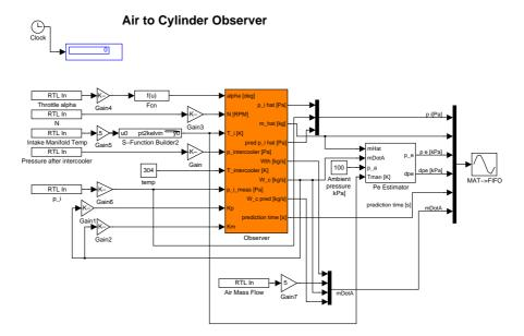
Figure 4.7: A model estimating the air-mass flow to the cylinder.
