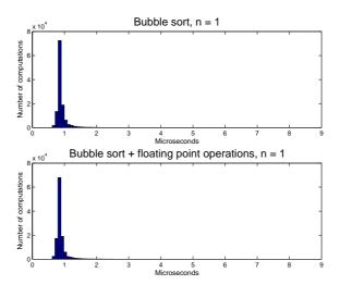
Figure 4.3: Histograms showing the variation of computation times needed for the algorithms bubble sort and bubble sort with floating point operations; where n = 1, sample time = 0.001 seconds, and the duration of the test =  $\sim$ 2 minutes.
