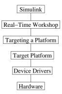
Figure 3.1: A way of viewing the system components and their relations to each other. Target platforms will be RTLinux or RTAI. The targeting of a platform is the conforming of the automatically Real-Time Workshop generated code to a specific platform.
