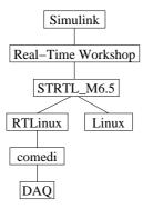
Figure 3.4: System overview with RTLinux as the hard realtime execution component and STRTL\_M6.5 as the component conforming the automatically Real-Time Workshop generated code to be runnable on RTLinux.
