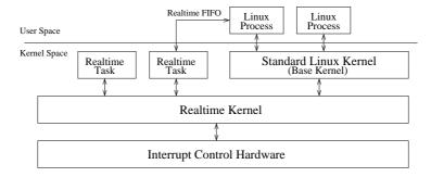
Figure 2.3: Flow of data and control. Ordinary Linux processes executes in user space, a protected environment, while the Linux kernel and the realtime tasks executes in kernel space, without protection against programming errors. Linux processes and realtime tasks communicates, e.g., via realtime FIFOs.
