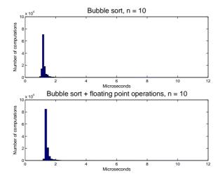
Figure 4.4: Histograms showing the variation of computation times needed for the algorithms bubble sort and bubble sort with floating point operations; where n=10, sample time = 0.001 seconds, and the duration of the test =  $\sim$ 2 minutes.
