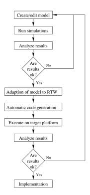
Figure 2.1: Rapid prototyping development process.
