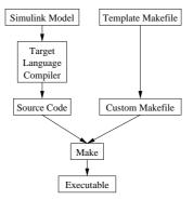
Figure 3.3: In the build process the Target Language Compiler generates source code, and a custom makefile is generated from the template makefile. To create the executable, the make -f model.mk command is issued.
