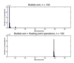
Figure 4.5: Histograms showing the variation of computation times needed for the algorithms bubble sort and bubble sort with floating point operations; where n=100, sample time = 0.001 seconds, and the duration of the test =  $\sim$ 2 minutes.
