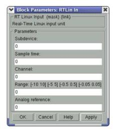
Figure 3.11: The input device driver block interface. Using the NI 6035e card: the *Subdevice* 0 is the group of analog input signals; in *Channel* the wanted input signal is chosen from the range [0 15], i.e. the card can handle 16 analog input signals; in *Range* there are 4 measurement ranges to choose among.
