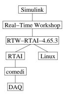
Figure 3.7: System overview with RTAI as the hard realtime execution component and RTW-RTAI-4.65.3 as the component conforming the automatically Real-Time Workshop generated code to be runnable on RTAI.
