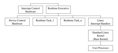
Figure 2.2: The structure of RTLinux. The realtime executive has no superior control of the interrupt control hardware implying the hardware latencies solely depend on the hardware. Linux itself is executing as a thread with the lowest priority, and all interrupts in the Linux interrupt handlers are soft interrupts, making Linux completely preemptible
