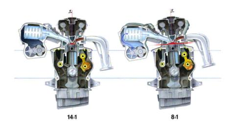
Figure 3.2: Showing the SAAB implementation of the SVC engine in the states of compression ratio 14 and 8.
