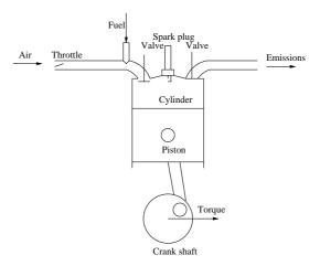
Figure 2.1: An engine takes air and fuel as input and generates torque and emissions.
