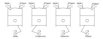
Figure 2.2: The four strokes intake, compression, expansion and exhaust of a four stroke engine.
