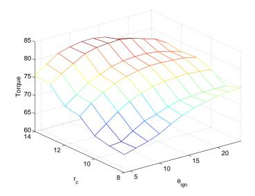
Figure A.3: Measurements of torque as a function of compression ratio and ignition angle, at working point 80 Nm and 2000 rpm
