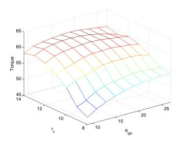
Figure A.2: Measurements of torque as a function of compression ratio and ignition angle, at working point 60 Nm and 2000 rpm
