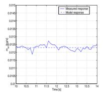
Figure 4.10: The air mass flow response for a compression ratio step at  $2000 \ rpm$ .
