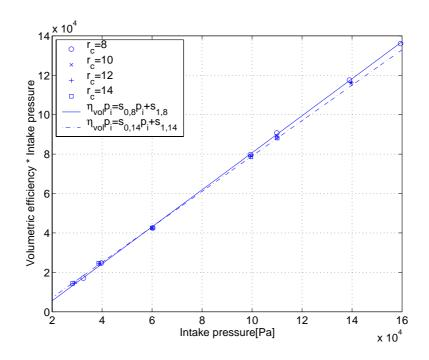
Figure 4.3: Shows  $\eta_{vol} \cdot p_i$  plotted against  $p_i$  for different compression ratios.
