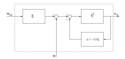
Figure 6.3: A block diagram of the controller.
