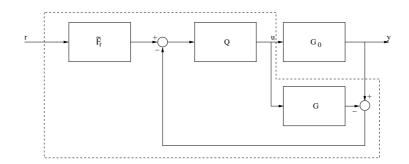
Figure 6.2: Feedback from model error.
