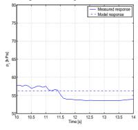
Figure 4.11: The intake pressure response for a compression ratio step at  $2000 \ rpm$ .
