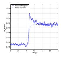
Figure 4.6: The air mass flow response for an air mass flow step at  $2000 \ rpm$ .
