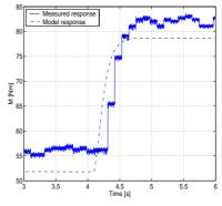
Figure 4.8: The torque response for an air mass flow step at  $2000 \ rpm$ .
