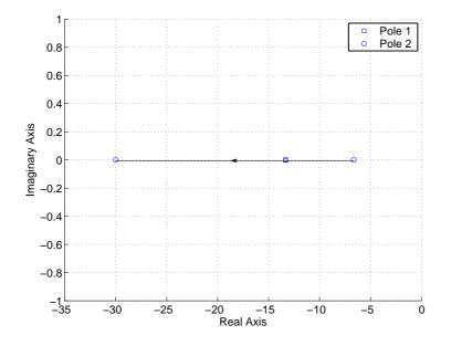
Figure 5.1: A plot that shows how one of the poles moves with different engine speeds, that pole is marked with a circle and moves from right to left along the real axis as the engine speed increases. The engine speed changes from 1000 rpm to 4500 rpm. The other pole, independent of operating characteristics, is marked with a square.
