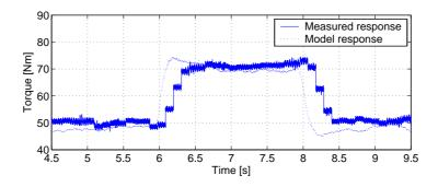
Figure 6.6: Shows measured torque and the estimated torque response for a air mass flow step at  $2000 \ rpm$ .
