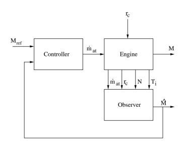
Figure 6.4: The observer estimates the torque from measurable signals and feedback the estimated torque to the controller.
