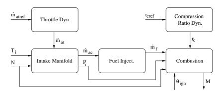
Figure 4.4: Input and output signals from engine subsystems and the interconnection between them.
