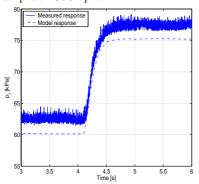
Figure 4.7: The intake pressure response for an air mass flow step at 2000 *rpm*.
