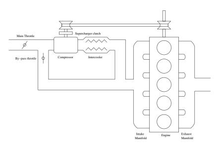
Figure 4.1: Sketch of the SVC engine. The figure illustrates how the engine is divided into subsystems to enable physical modeling of the engine.
