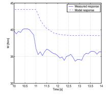
Figure 4.12: The torque response for a compression ratio step at  $2000 \ rpm$ .
