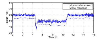
Figure 6.5: Shows measured torque and the estimated torque response for a compression ratio step from 14 to 8 and 8 to 14 at 2000 *rpm*.
