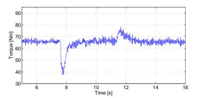
Figure 6.7: Torque measurements of how the controller handles a compression ratio step from 14 to 8 and 8 to 14 at 2000 rpm.
