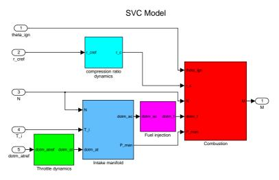
Figure C.1: The figure shows the top level of the SIMULINK model.
