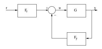
Figure 2.3: A controller with two degrees of freedom.
