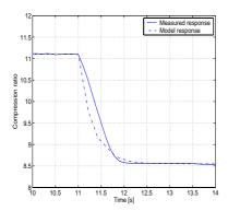
Figure 4.9: The compression ratio response for a compression ratio step at  $2000 \ rpm$ .
