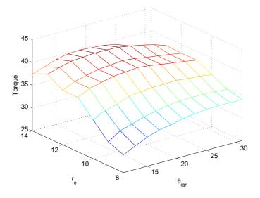
Figure A.1: Measurements of torque as a function of compression ratio and ignition angle, at working point 40 Nm and 2000 rpm
