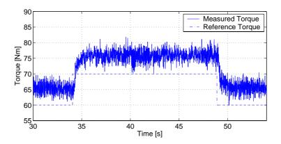
Figure 6.8: Torque measurements of how the controller handles a torque reference step from 60 Nm to 70 Nm and 60 Nm to 70 Nm at 2000 rpm.
