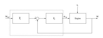
Figure 6.1: Showing the control structure used. The box surrounds the blocks that belong to the controller. The figure also shows important signals.
