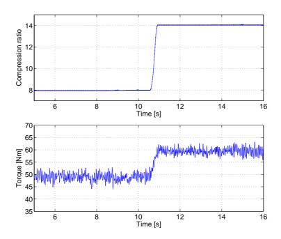
Figure 1.1: Shows how the output torque changes when the compression ratio changes from 8 to 14, at 2000 *rpm*. The top plot shows the compression ratio and the bottom plot shows the output torque.
