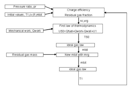
Figure 5.5: Flowchart over the algorithm with  $m_{rq}$
