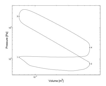
Figure 2.1: Volume vs Pressure in a conventional spark ignited engine in a log-log diagram
