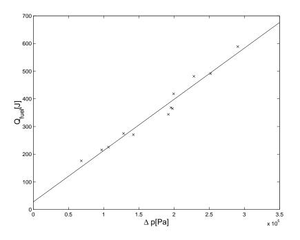
Figure 5.2: Correlation between  $\Delta p_{comb}$  and  $Q_{fuel}$
