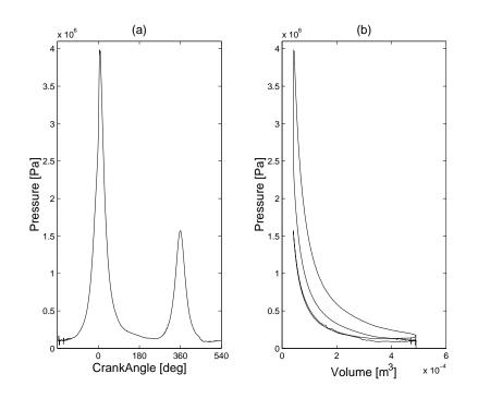
Figure 4.1: Crankangle vs Pressure (a) and Volume vs Pressure (b)
