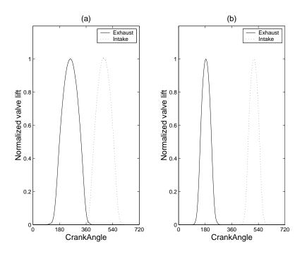
Figure 3.1: Normalized valve lift for an SI-engine(a) and an HCCI-engine(b)
