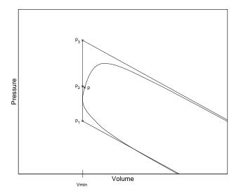
Figure 4.2: Definition of the points used for mass fraction burned calculation
