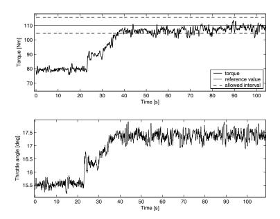
Figure 7.7: Case one. Torque and throttle angle during the whole control time.
