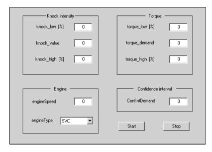
Figure 5.1: The GUI used to manage the knock intensity and torque controller.
