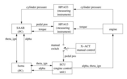
Figure 6.2: A schematic picture of the components that are used in the laboratory.
