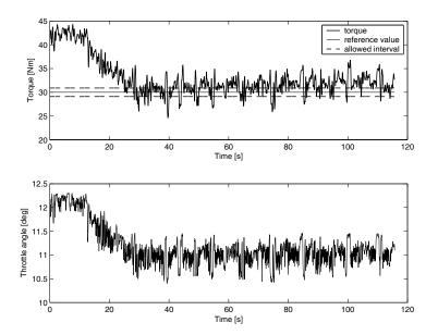
Figure 7.15: Case three. Torque and throttle angle for the whole control time.
