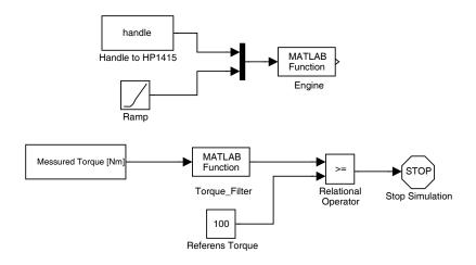
Figure 5.3: The Simulink model that handles the torque ramping.
