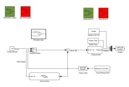
Figure 4.4: The Simulink model used for knock intensity and torque control.
