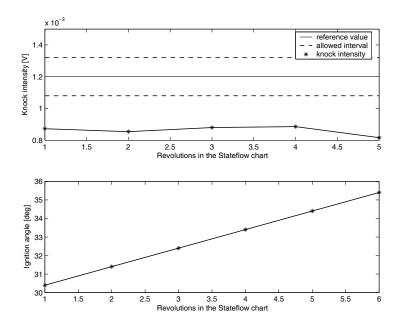
Figure 7.13: Case three. Knock intensity and ignition angle.
