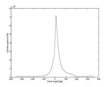
Figure 2.2: The cylinder pressure plotted against the crank angle.
