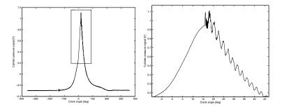
Figure 2.3: A cylinder pressure curve with knock. The left plot shows a whole cycle and the right plot shows an enlargement of the area of interest.
