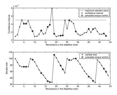
Figure 7.17: Confidence interval and sample size when the controller is run from the script.
