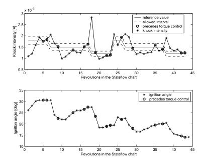
Figure 7.16: Knock intensity and ignition angle when the controller is run from the script. After revolution 23 the reference torque is changed from 90 to 110 Nm.
