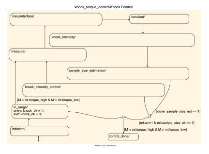
Figure 4.3: A stripped version of the knock intensity control Stateflow chart.
