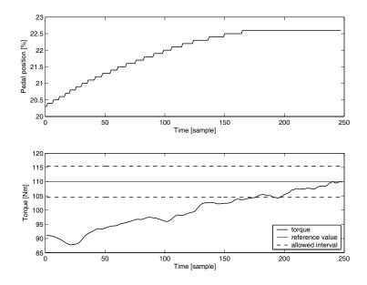
Figure 7.4: Case one. Torque and pedal position during the torque control.
