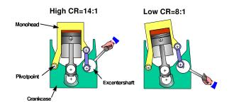
Figure 2.7: A schematic description of variable compression.
