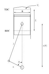
Figure 2.1: Some important parameters in the cylinder geometry.
