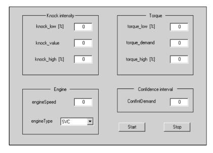
Figure C.1: The GUI used to manage the knock and torque regulator.
