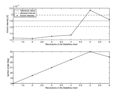
Figure 7.5: Case one. Knock intensity and ignition angle.
