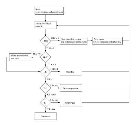
Figure 5.2: A flow diagram describing how the script iterates through all operating points and avoids those with to high knock. THK and TLK are short for To High Knock and To Low Knock respectively. I.K, C.I and TI are short for Index of Knock, Compression Index and Torque Index.
