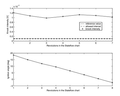
Figure 7.9: Case two. Knock intensity and ignition angle.
