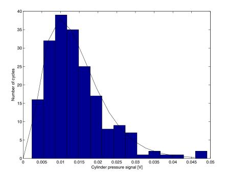
Figure 3.1: A histogram of the measured data from one operating point containing 200 cycles. Shown in the plot is also the Gamma distribution that gives the best fit.
