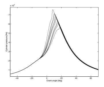
Figure 2.4: Cycle to cycle variations for ten consecutive cycles when all the controllable parameters are held constant.
