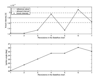
Figure 7.1: Knock intensity and ignition angle. The thin line is the goal value and the dashed lines is the accepted range.
