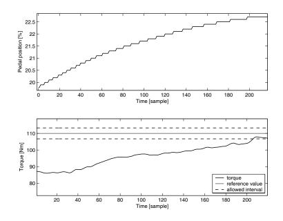
Figure 7.8: Case two. Torque and pedal position during the torque control.
