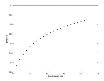
Figure 2.6: Engine efficiency as a function of the compression ratio. This shows the ideal case when heat transfer is not taken into consideration.
