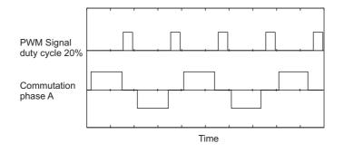
Figure 6.4: Problems occur when the commutation and the PWM signal have the same frequency. In this case will phase A always be low.
