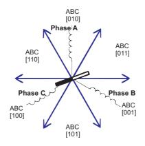
Figure 3.3: The six hall sensor states of the motor.
