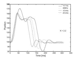
Figure 6.3: Comparison between four different PWM frequencies. Both the low and the high frequencies have problems.
