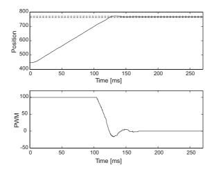
Figure 5.3: A step where the control signal is turned off after the position has been in the right area for 100 samples. The position at the y-axis is referring to the number of hall state changes.
