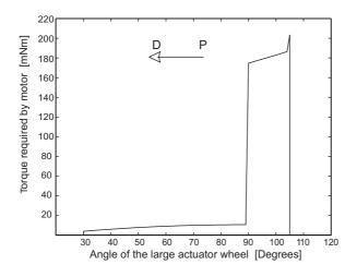
Figure 2.3: The torque characteristics when shifting from P to D. P is at  $105^{\circ}$  and D is at  $20^{\circ}$ .
