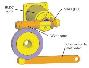
Figure 2.2: Actuator: DC motor and a gear reduction of 1:200.
