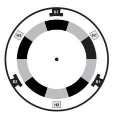
Figure 3.9: The MMT motor with five polepairs.
