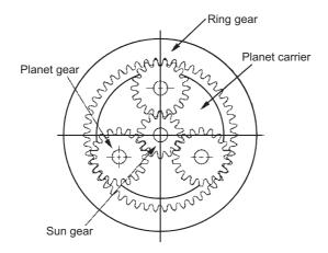
Figure 2.1: A planetary gear system.
