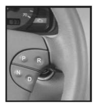
Figure 1.1: Shift control at the steering wheel. A possibility with Shiftby-Wire.
