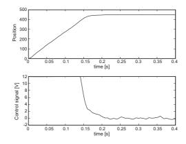
Figure 4.4: The results from a simulation with K=0.5 and  $T_d=0.004$ . The y-axis in the position plot is scaled to match the hall state changes.
