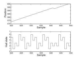
Figure 5.6: An error occurs in the hallstate counter function at sample 642.
