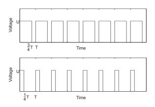
Figure 3.2: PWM signals with 75% and 25% duty cycle respectively.
