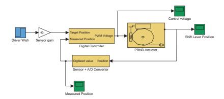
Figure 4.1: A model of the total system.
