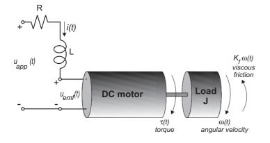
Figure 4.2: A simple model of a DC motor.
