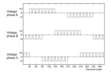
Figure 3.8: Voltages for each phase from the bridge gate driver.
