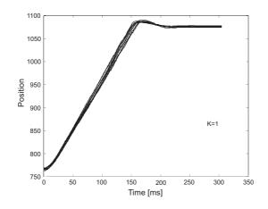
Figure 6.2: A shift from N to D using 8 different PWM frequencies.
