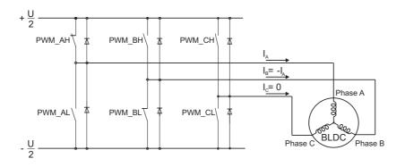
Figure 3.6: An example of a three phase bridge gate driver that handles the current supply to the motor. In this case  $PWM_{AH}$  and  $PWM_{BL}$  are high.
