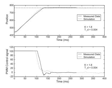
Figure 6.1: Comparison between the simulink model and measured data.
