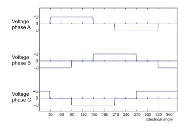
Figure 3.5: Voltage strokes applied for counterclockwise rotation.
