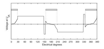
Figure 3.11: Branch voltage during one revolution. The angular position of the rotor can be estimated by sensing the zero-crossing points, here at  $180^{\circ}$  and  $360^{\circ}$ .
