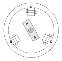
Figure 3.1: A three-phase BLDC motor.
