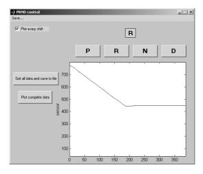
Figure 5.2: A screen shot of the Matlab Graphical User Interface that receives data from the SCU via the serial port.
