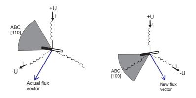
Figure 3.4: The commutation process. The left figure shows the moment prior to commutation and the right the situation afterwards for rotation counterclockwise.
