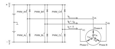
Figure 3.10: The three phase bridge driver with the back-EMF voltages  $u_{iA}$ ,  $u_{iB}$  and  $u_{iC}$  shown.
