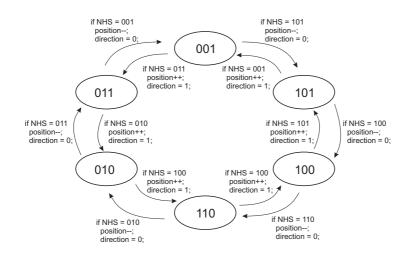
Figure 5.5: The principle for the hall state change counter function. NHS = New Hall State.
