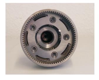
Figure 2.5: The 45RFE Planetary Gear Set without the Sun Gear
