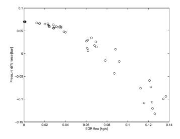
Figure 4.3: Pressure difference vs. EGR flow.
