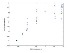
Figure 5.3: Measured effective area (o) and modelled effective area (x) for the single restriction black-box model
