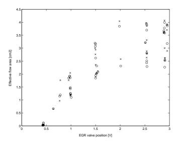
Figure 4.2: Measured effective area (o) and fitted model data (x), black-box model.
