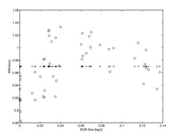
Figure 4.6: Measured cooler efficiency (o) and fitted model data (x).
