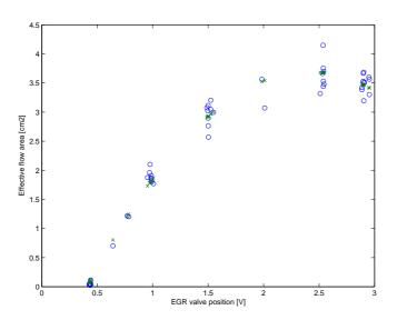
Figure 4.4: Measured effective area (o) and fitted model data (x), two stage restriction model.
