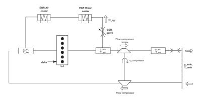
Figure 3.6: Extended model with single restriction EGR model.
