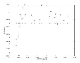
Figure 5.9: Measured efficiency (o) and modelled efficiency (x) for the air cooler.
