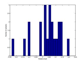
Figure 5.4: Histogram of the relative errors for the black-box model.
