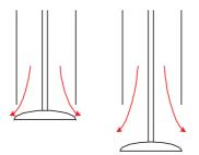
Figure 3.4: Illustrating the linear and evening-out phase of the effective flow area.
