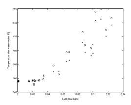
Figure 5.8: Measured temperature after the water cooler (o) and modelled temperature (x).
