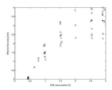
Figure 4.1: Measured effective area (o) and fitted model data (x), polynomial model.
