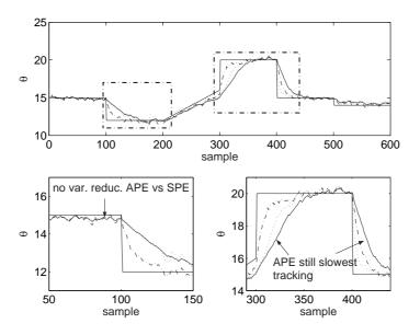
Figure 4.8. Estimator with adaptive center and static sigma. APE shows little or no variance reduction vs. SPE but still slower response time. APE estimates solid, SPE dotted and LP-filter dash-dotted.
