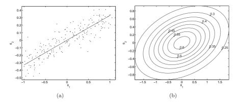
Figure 4.10. (a) Correlation of two variables from a hypothetical experiment. The line shows the actual relationship between the variables. (b) A contour plot of a 2D PDF of two variables with linear correlation. Contours marked with corresponding probability density.
