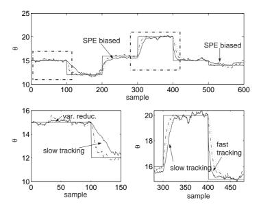
Figure 4.5. Tracking over large steps. SPE solid, LP estimate dash-dotted, bootstrap estimate dotted. Settings:  $\mu_p = 15$ ,  $\sigma_p = 1$ , noise  $\sigma_{\theta} = 1$ , LP-factor= 0.90, min(Prior)= 0.1
