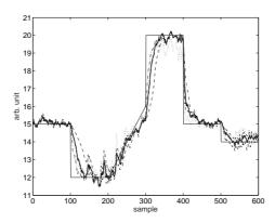
Figure 4.3. Tracking plot with the various weighting functions. LP-filter (dasheddotted) and hit-or-miss (dotted) are fastest and inverse quadratic (dashed) slowest tracking while all others, (solid), are in between.
