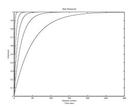
Figure 3.9. The step responses of the LP filter in (3.23). Forgetting factors  $a = \{0.5 \ 0.8 \ 0.9 \ 0.95 \ 0.98\}$ .
