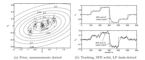
Figure 4.13. This track stays within probable area of the prior. Note the near match between the SPE and the LP-filter.
