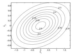
Figure 3.2. Contour plot of a gaussian 2d-prior. The contours represent constant probability density with the highest density in the middle. The inclination of the major axis represents the correlation between x and y.
