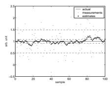
Figure 3.3. Example showing the concentration/reduced variance of the estimates when using an LP-filter. Dash-dotted lines represent the variance of the measurements and estimates respectively.
