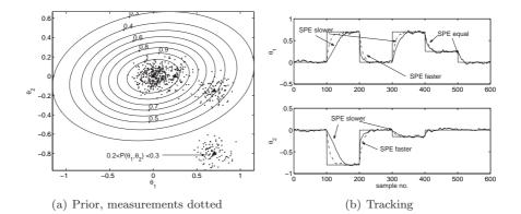
Figure 4.11. Note the reluctance to move away from a probable area at 100-200, the fast step towards a probable area at 200 and the difference in response at 300 and 100. Triangles in (a) correspond to the setpoints in (b).
