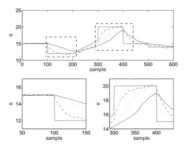
Figure 4.9. Estimator with adaptive center, adaptive sigma and LP-factor 0.95. Increasing the LP-factor further slows the APE estimate down. APE estimates solid, SPE dotted and LP-filter dash-dotted.
