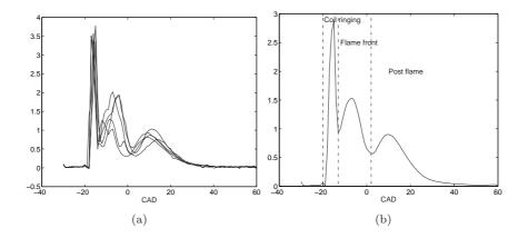
**Figure 2.3.** (a) Five ionization current measurements from consecutive cycles. (b) An ionization current curve averaged over 100 cycles. The three characteristic phases are easily visible: Coil ringing, flame front and post flame.
