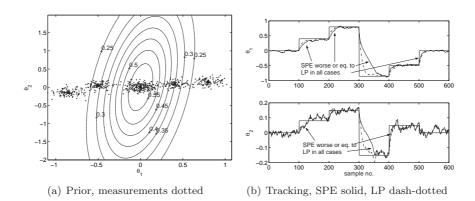
Figure 4.14. This track moves mainly in the improbable areas of the prior. Note that the LP filter performs better everywhere except at the step back to (0,0) at 500. Settings: Noise levels  $(\sigma_{\theta_1}, \sigma_{\theta_2}) = (0.1, 0.08)$ , prior  $\sigma = (0.1, 2)$ , LP-factor: 0.9, min(prior) = 0.2
