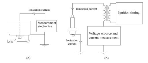
**Figure 2.2.** Measurement of the ionization current. (a) The spark plug-gap is used as a probe. (b) Measurement on the low voltage side. (Figure from Eriksson [11])
