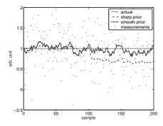
Figure 3.6. Stationary tracking with sharp prior vs. smooth prior. Prior biased after sample 100.
