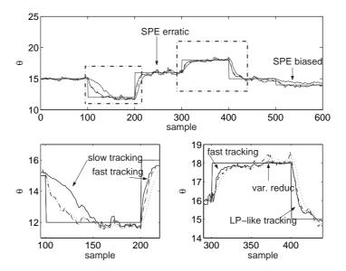
Figure 4.6. Tracking when using a bimodal prior. SPE solid and biased, LP estimate dashed, bootstrap estimate dotted.
