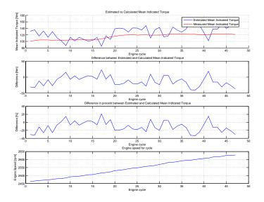
Figure 8.26: Estimated vs Calculated torque for third gear. TOP: Estimated and calculated mean indicated torque. TWO IN THE MIDDLE: Difference between the estimated and calculated torque in Nm and percent. BOTTOM: Engine speed.
