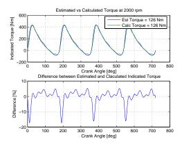
Figure 8.11: Estimated and Calculated Instantaneous Indicated Torque
