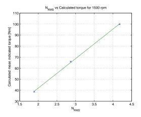
Figure 8.15: N<sub>RMS</sub> vs Calculated Mean Indicated Torque
