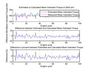
Figure 8.19: Estimated and Calculated Mean Indicated Torque for 2500 rpm
