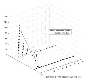
Figure 6.2: Comparison between DFT of Crankshaft Speed and Indicated Torque
