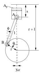
Figure 3.1: The crank-slider mechanism
