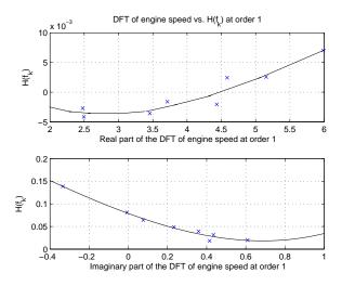
Figure 8.10: DFT of Engine Speed vs  $\hat{H}$  at order 1 and 3500 rpm
