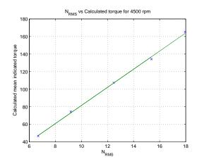
Figure 8.17: N<sub>RMS</sub> vs Calculated Mean Indicated Torque
