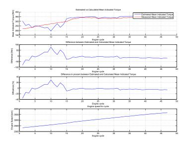
Figure 8.25: Estimated vs Calculated torque for second gear. TOP: Estimated and calculated mean indicated torque. TWO IN THE MIDDLE: Difference between the estimated and calculated torque in Nm and percent. BOTTOM: Engine speed.
