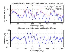
Figure 8.2: Estimated and calculated torque at 2500 rpm.
