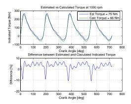
Figure 8.12: Estimated and Calculated Instantaneous Indicated Torque
