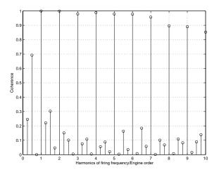
Figure 6.4: Coherence function for the DFT of the Crankshaft Speed and the Instantaneous Indicated Torque
