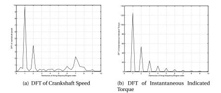
Figure 6.3: Illustration of the DFT of the Crankshaft Speed and the Instantaneous Indicated Torque with the mean value of the signal removed.
