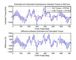
Figure 8.3: Estimated and calculated torque at 4000 rpm.
