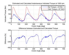
Figure 8.1: Estimated and calculated torque at 1000 rpm.
