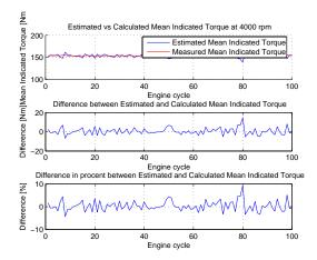
Figure 8.20: Estimated and Calculated Mean Indicated Torque for 4000 rpm
