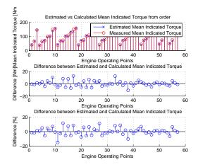
Figure 8.21: Estimated and Calculated Mean Indicated Torque for all engine operating points
