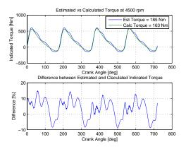
Figure 8.13: Estimated and Calculated Instantaneous Indicated Torque
