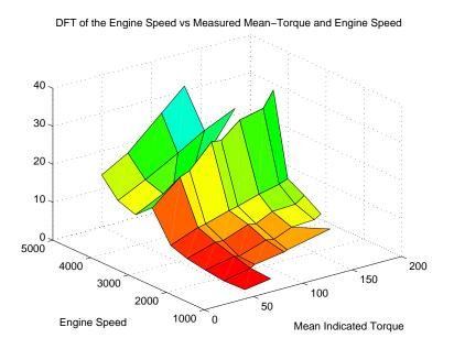
Figure 8.14: DFT of the Engine Speed vs Calculated Indicated Torque and Engine Speed.
