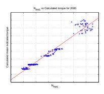
Figure 8.24:  $N_{RMS}$  vs Calculated torque for 2000 rpm and fourth gear
