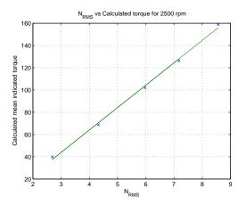
Figure 8.16:  $N_{RMS}$  vs Calculated Mean Indicated Torque
