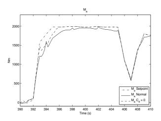
Figure 5.21: Torque when  $C_4=0$ , i.e. low weight on  $\lambda$  compared with the normal weight.
