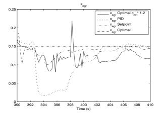
Figure 5.33:  $x_{egr}$  with  $c_{m1} \cdot 1.2$  compared to normal  $x_{egr}$  and  $x_{egr}$  for the PID controller.
