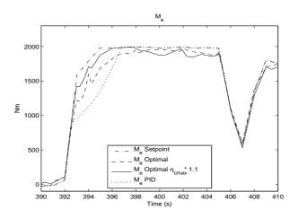
Figure 5.35:  $M_e$  with a higher maximal efficiency on the compressor compared to the normal efficiency.
