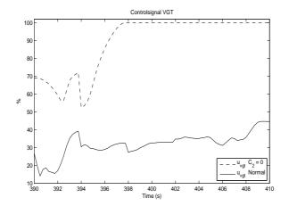
Figure 5.13: VGT when  $C_2=0$ , i.e. low weight on  $x_{egr}$  compared with the normal weight.
