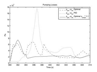
Figure 5.34: Pump losses with a higher maximal efficiency on the compressor compared to the normal efficiency.
