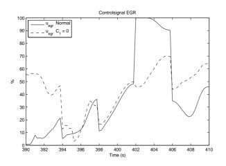
Figure 5.23: EGR when  $C_1=0$ , i.e. low weight on  $u_{\delta}$  compared with the normal weight.
