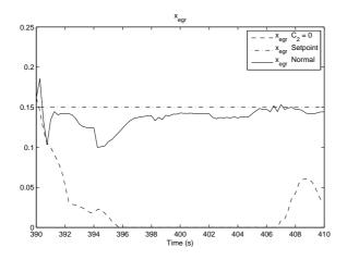
Figure 5.16:  $x_{egr}$  when  $C_2=0$ , i.e. low weight on  $x_{egr}$  compared with the normal weight.
