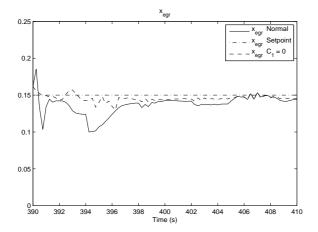
Figure 5.26:  $x_{egr}$  when  $C_1=0$ , i.e. low weight on  $u_{\delta}$  compared with the normal weight.
