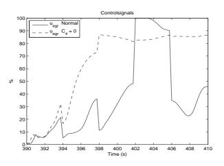
Figure 5.18: EGR when  $C_4=0$ , i.e. low weight on  $\lambda$  compared with the normal weight.
