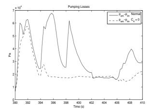
Figure 5.20: Pump losses when  $C_4=0$ , i.e. low weight on  $\lambda$  compared with the normal weight.
