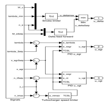
Figure 3.1: Simulink model of the PID structure
