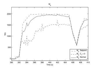
Figure 5.27: Torque when  $C_1=0$ , i.e. low weight on  $u_{\delta}$  compared with the normal weight.
