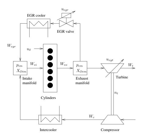
Figure 2.1: The structure of the diesel engine model.
