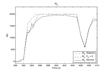
Figure 5.15: Torque when  $C_2=0$ , i.e. low weight on  $x_{egr}$  compared with the normal weight.
