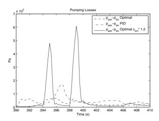
Figure 5.32: Pump losses with  $c_{m1} \cdot 1.2$  compared to normal pump losses and pump losses for the PID controller.
