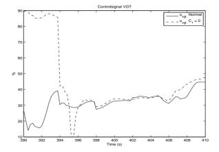
Figure 5.24: VGT when  $C_1=0$ , i.e. low weight on  $u_{\delta}$  compared with the normal weight.
