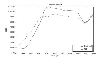
Figure 5.7: Turbine speed from the optimal control signals and from the PID-controller.
