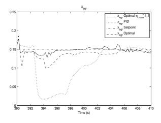
Figure 5.37:  $x_{egr}$  with a higher maximal efficiency on the compressor compared to the normal efficiency.
