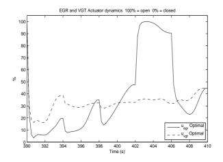
Figure 5.5: The states of the optimal EGR and VGT signals.
