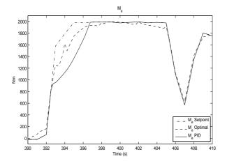
Figure 5.10: The torque from the optimal control signals and from the PID controller.
