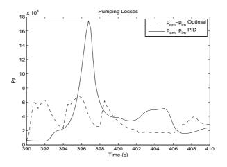
Figure 5.11: Pump losses from the optimal control signals and from the PID controller.
