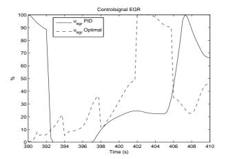
Figure 5.3: The optimal EGR signal and the EGR signal from the PID simulation.
