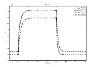
Figure 4.1: Step response in  $P_{im}$  and  $P_{em}$  for the original simulink model and the model implemented in TOMOC
