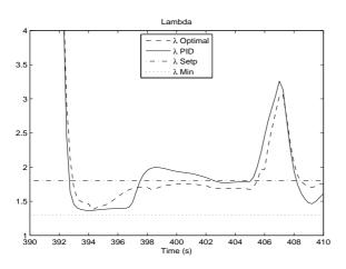
Figure 5.9:  $\lambda$  from the optimal control signals and  $\lambda$  from the PID-controller compared to the set point and to  $\lambda_{min}$ .
