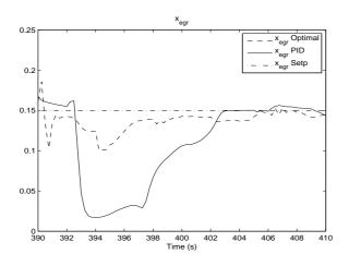
Figure 5.6: The EGR mass fraction from the optimal control signals and from the PID-controller compared to the set point.
