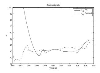
Figure 5.4: The optimal VGT signal and the VGT signal from the PID simulation.
