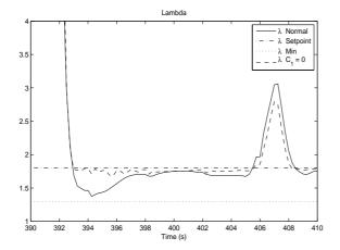
Figure 5.28:  $\lambda$  when  $C_1=0$ , i.e. low weight on  $u_{\delta}$  compared with the normal weight.
