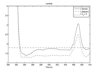
Figure 5.17:  $\lambda$  when  $C_2{=}0,$  i.e. low weight on  $x_{egr}$  compared with the normal weight.
