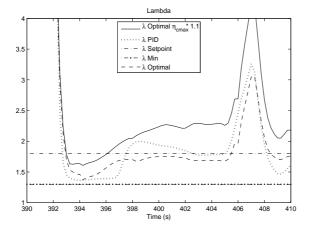
Figure 5.36:  $\lambda$  with a higher maximal efficiency on the compressor compared to the normal efficiency.
