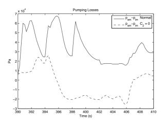
Figure 5.14: Pump losses when  $C_2=0$ , i.e. low weight on  $x_{egr}$  compared with the normal weight.
