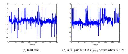
Figure 8.13: The residual in EGR-flow test.
