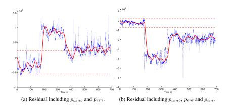
Figure 8.15: Residuals during pressure adaption. The fault in  $p_{amb}$  occurs after 180s. Then the adaption is simulated so after 370s,  $p_{im}$  and  $p_{em}$  are adapted.
