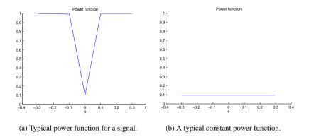
Figure 5.1: Two different power functions for residuals in the automatic designed OBD-system.
