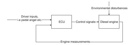
Figure 3.2: Principle of engine with control system.
