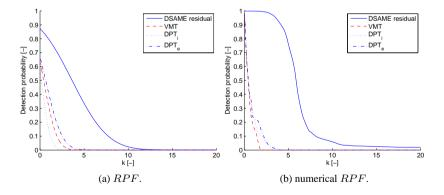
Figure 8.5: Residual performance for 30% gain fault in  $p_{em}$ .
