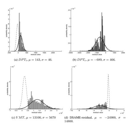
Figure 8.3: Comparison of measured histogram and the power density function from estimated  $N(\mu, \sigma)$  for residuals when  $p_{im}$  is stuck. The dashed lines are the distributions from the fault free case for each residual.
