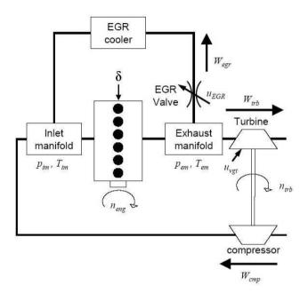
Figure 3.1: Schematic figure of the gasflow of a diesel engine with VGT and EGR.
