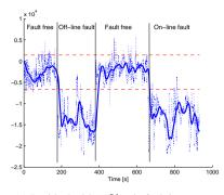
(a) Residual with 30% gain fault in  $w_{cmp}$ .
