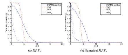
Figure 8.4: Residual performance for 30% gain fault in  $p_{im}$ .
