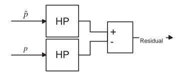
Figure 4.2: Schematic figure over the principle for the dynamic pressure tests.
