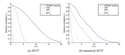
Figure 8.6: Residual performance when  $p_{im}$  is stuck.
