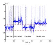
(b) Residual with 30% gain fault in  $p_{em}$ .
