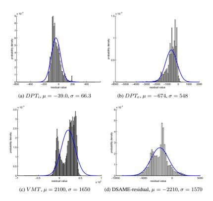
Figure 8.1: Comparison of measured histogram and the power density function from estimated  $N(\mu, \sigma)$  for fault free residuals.
