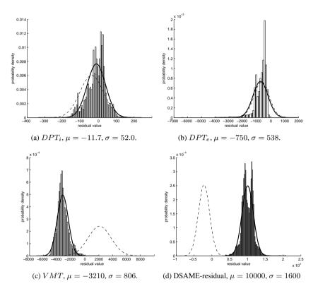
Figure 8.2: Comparison of measured histogram and the power density function from estimated  $N(\mu, \sigma)$  for residuals with 30% gain fault in  $p_{im}$ . The dashed lines are the distribution from the fault free case for each residual.
