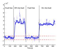
(c) Residual with 30% gain fault in  $p_{im}$ .
