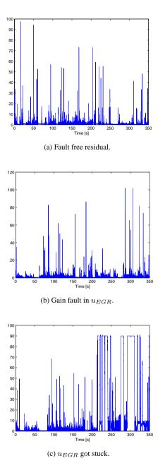
Figure 8.11: The residual for EGR-damper test with different fault-simulation. The faults are added at time=220s.
