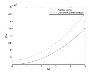
Figure 7.1: By changing the electrical curve a fault can be simulated.
