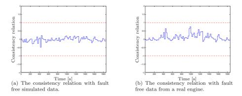
Figure 5.4: The consistency relation with no fault added with simulated and real data. Both consistency relations have been scaled equally much.
