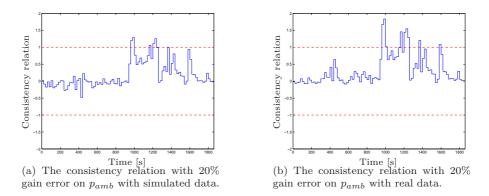
Figure 5.5: The consistency relation with 20% gain fault on  $p_{amb}$  with simulated and real data. Both consistency relations have been scaled equally much.
