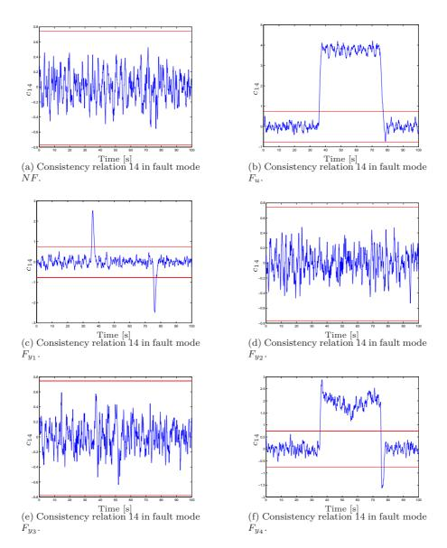
Figure 3.5: Consistency relation 14 with faults.
