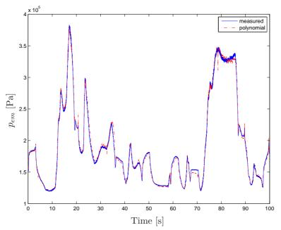
Figure 5.1: The pressure in the exhaust manifold,  $p_{em}$ , as measured (solid) values and simulated with polynomials (dash-dotted).
