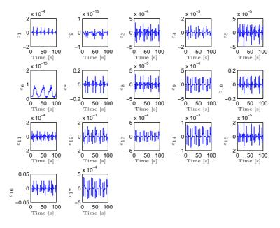
Figure 3.4: The consistency relations in the fault free case with no measurement noise added.
