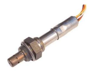
Figure 1.5: The Figure shows one of the most important sensor in a modern car, the lambda sensor. It was designed to sense the (A/F)-ratio so an effective feedback loop could be implemented in todays fuel injections. (courtesy of David Long [12])
