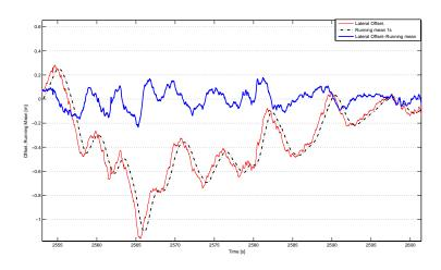
Figure 5.2. The calculation of the deviation from the current driving trajectory, normal straight ahead driving. The dotted line is the moving average over 1s and the thin solid line is the lateral offset signal. The result of the calculation (i.e. the difference between the offset and the moving average) is depicted as the thick solid line.
