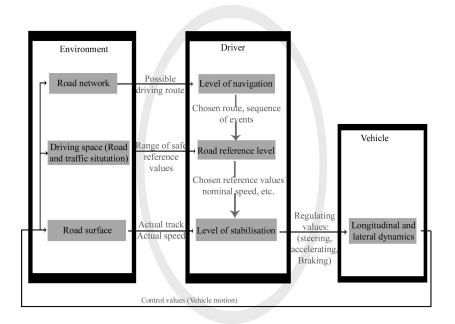
Figure 2.2. Hierarchical 3-Level structure showing the task of driving a car (from Donges, 1982 in [7]). Highlighted is the part which applies to the driver perspective.
