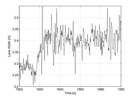
Figure 3.3. Lane width signal from the lane monitoring system.
