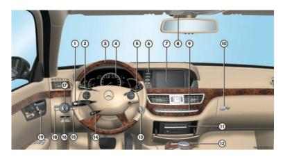
Figure 2.3. Operating elements in the driving seat. Number 12 points at the area where the COMAND controller and the number pad is situated. Number 7 points at the Comand display. ©DaimlerChrysler
