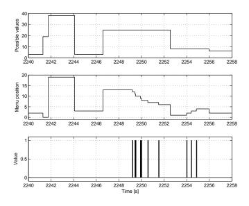
Figure 5.6. Example of state signals, the COMAND controller. From the top are the possible menu values, the current menu position and the resulting OE signal.
