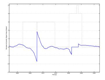
Figure 5.4. Filtering out the lane changes and the spikes. The solid line represents the lateral offset signal and the dotted signal shows where the lane changes and the spikes were detected and how much of the signal was filtered out in the calculation. When the dotted signal in the figure is  $\geq 0$  the Overridden Area is not summed up.
