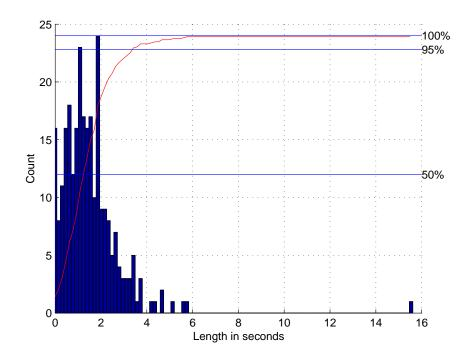
Figure 6.3. Figure showing a histogram over the pauses between the task operating parts of task 3, number pad. Blue lines show the level where the probability density function (thin curve) is 50%, 95% and 100%.
