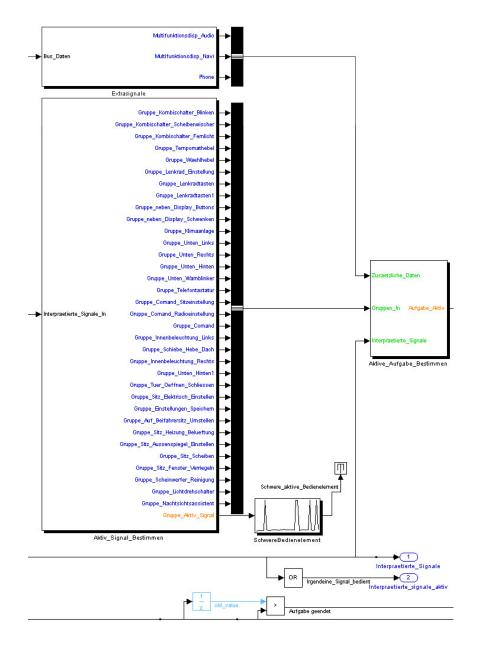
Figure 5.7. The part of the model which contains the task-, active task and group selection.
