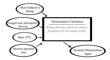
Figure 7.1. Overview of the possible and current inputs to the current driver distractedness model.
