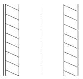
Figure 2.1: Lane with VEZs. Broken line designates lane center. [Observe that the VEZs are not drawn in scale.]
