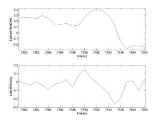
Figure 7.1: Above: Lateral offset of the vehicle. [Offset in meters] Below: Lateral velocity of the vehicle derived from lateral offset. [Velocity in meters/second]
