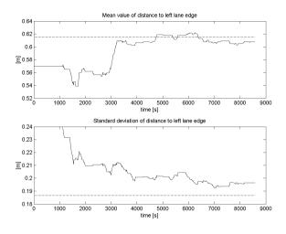
Figure 4.1: Comparison between real and approximated mean value and standard deviation. Calculated over distances to left lane edge. The broken line shows the values calculated over all samples in the test drive.
