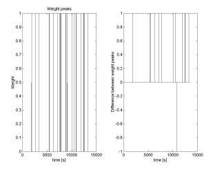
Figure 4.4: Weight peaks generated during system simulation with and without constant offset. Left: Weight peaks plotted in the same figure. Right: Difference between the plotted weight peaks.
