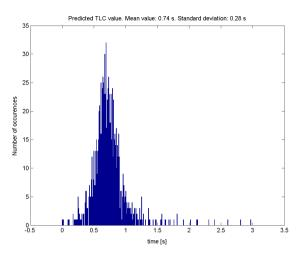
Figure 8.3: TLC predicted by the TLC system. Real TLC is 0.6 seconds. [Cases where TLC prediction is 3 seconds, i.e. cases where predicted TLC is undefined, are not shown. They are 4% of the cases]
