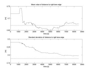
Figure 4.2: Comparison between real and approximated mean value and standard deviation. Calculated over distances to right lane edge. The broken line shows the values calculated over all samples in the test drive.
