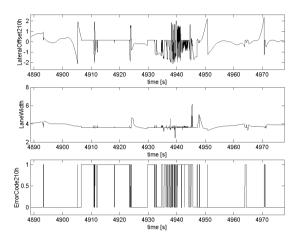
Figure 3.3: Signals from the LDS. Typical signal characteristics when error signal is 1. [Offset and lane width in meters]
