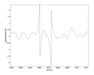
Figure 3.1: Lateral offset signal from the LDS. Typical signal characteristics when overtaking. Lane change to the left are followed by lane change to the right. [Offset in meters]
