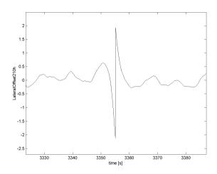
Figure 2.2: Lateral offset signal from the LDS. Typical lane change to the right. [Offset in meters]
