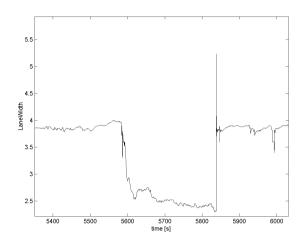
Figure 2.3: Lane width signal from LDS. Lane width while passing a construction site. [Lane width in meters]
