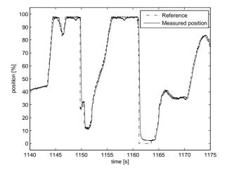
Figure 6.19. Reference for the piston position from a common driving case and measured piston position in an engine test cell with On/Off valves.
