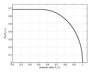
Figure 2.11. The function  $\Psi$ , depending on upstream to downstream pressure ratio. When  $P_r$  is greater than 0.99  $\Psi$  is approximated with a linear function.
