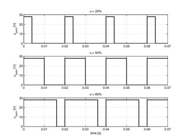
**Figure 2.3.** Simulated PWM signals with period time T = 20 ms where  $u_{pwm} = 28$  V represents high and  $u_{pwm} = 0$  V represents low. From top to bottom: u = 20%, u = 50% and u = 80%.
