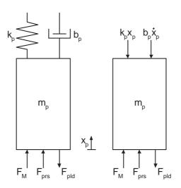
Figure 2.9. Sketch and free body diagram of the plunge.
