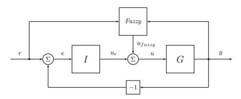
Figure 6.5. The structure of the fuzzy-I controller implemented in simulation.
