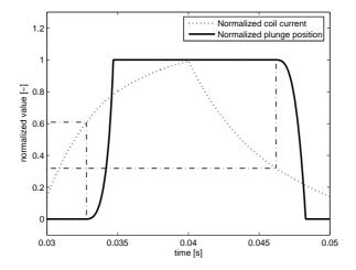
Figure 5.2. Simulation of the current through the coil and the plunge movement, showing at which current levels the plunge starts to move.
