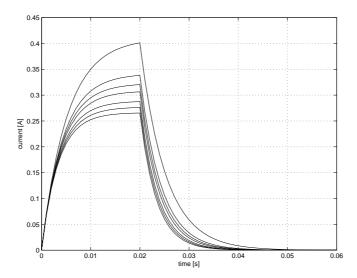
Figure 5.3. Simulated current in the electric circuit at different temperatures. From top to bottom:  $0^{\circ}$ C,  $20^{\circ}$ C,  $40^{\circ}$ C,  $60^{\circ}$ C,  $80^{\circ}$ C,  $100^{\circ}$ C and  $120^{\circ}$ C.
