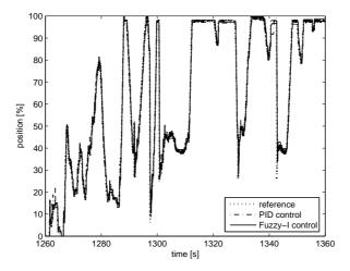
Figure 6.13. A reference for the EGR valve with the simulated output retrieved with a PID controller and a fuzzy-I controller.
