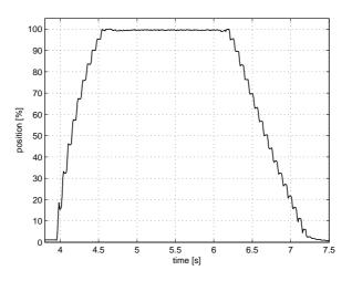
Figure 5.7. Different measured lengths in movement when increasing the piston position, dependent on start position. Constant length when decreasing it.
