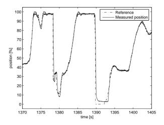
Figure 6.20. Reference for the piston position from a common driving case and measured piston position in an engine test cell with the EGR valve control system used today.
