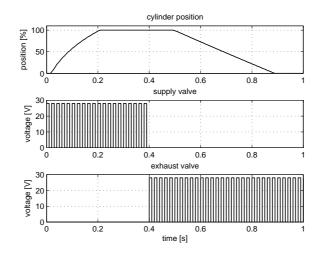
Figure 5.6. Measured piston position when given a constant input signal of 50% first to the supply valve, then to the exhaust valve, showing that the system is integrating.
