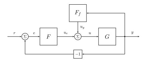
Figure 6.16. The structure of the controller implemented in the test bench.
