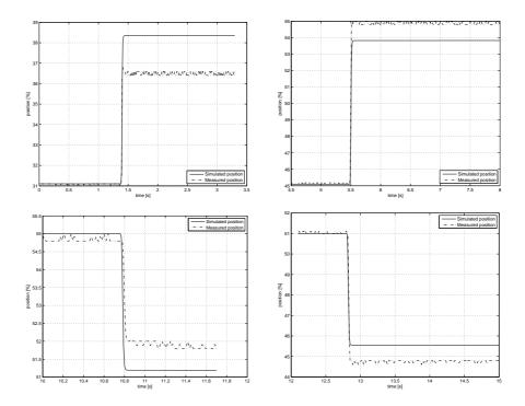
Figure 3.1. Examples of steps between two different levels used to calibrate the static parameters of the model.
