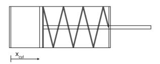
Figure 2.13. Schematic figure of the pneumatic cylinder.
