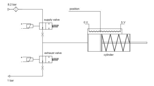
Figure 2.1. Overview of the system configuration with the two On/Off valves and the cylinder.
