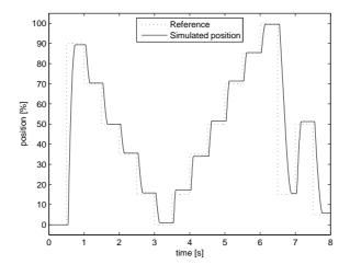
Figure 6.11. The pneumatic system simulated with a fuzzy controller.
