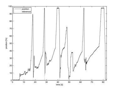
Figure 6.17. Reference for the piston position from a common driving case and measured piston position in a test bench.
