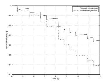
Figure 5.5. The pressure changes while the piston is at a constant position without any applied control signal. This shows the presence of thermodynamic effects.
