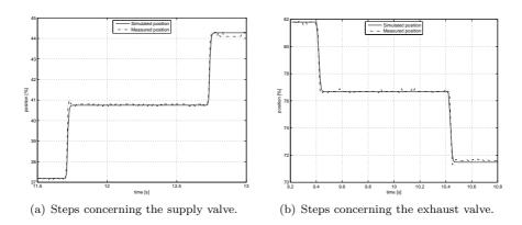
Figure 3.2. Examples of steps used to calibrate the dynamic parameters of the model.
