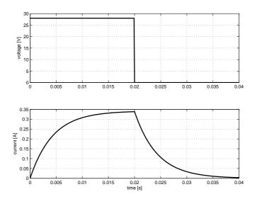
Figure 5.1. Simulation of the input voltage and the resulting current through the coil.
