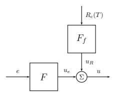
Figure 5.4. The basic structure of feedforward control from temperature.
