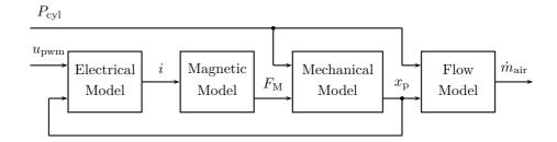
Figure 2.4. Block diagram of the valve.
