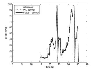
Figure 6.12. A reference for the EGR valve with the simulated output retrieved with a PID controller and a fuzzy-I controller.
