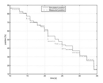
Figure 3.4. Simulated and measured position for the static calibration data for the exhaust valve.
