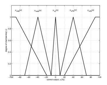
Figure 6.9. Suggested membership functions for the output signal.
