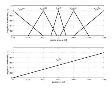
Figure 6.8. Suggested membership functions for the controller input.
