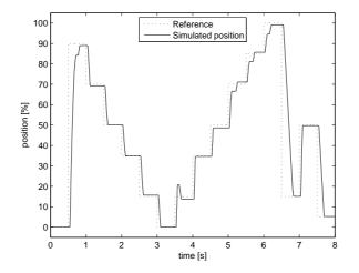
Figure 6.4. The pneumatic system simulated with a PID-controller.
