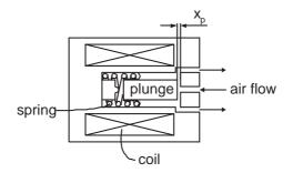
Figure 2.2. Sketch of the On/Off valve.
