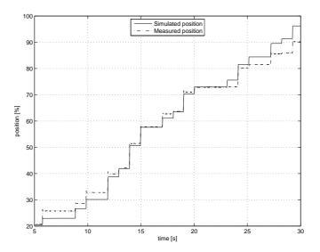
Figure 3.3. Simulated and measured position for the static calibration data for the supply valve.
