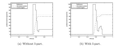
Figure 6.2. The difference between a controller with an I-part compared to one without in simulation.
