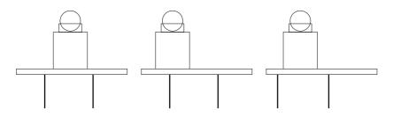
Figure 4.3: Three different ways of placing pistons in relation to the driver.
