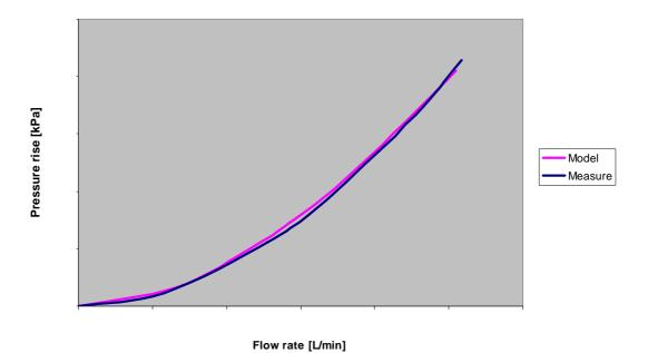
Figure 58. System curve, Test 11.
