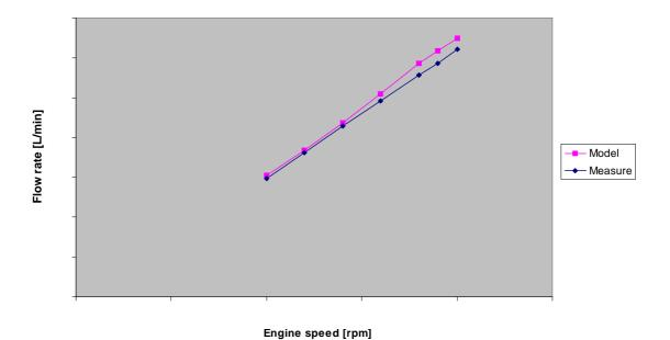
Figure 68. Flow through transmission oil cooler, Test 13.
