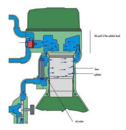
Figure 93. The flow through cylinder head and cylinder block.
