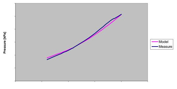
Figure 61. Pressure after coolant pump, Test 11.
