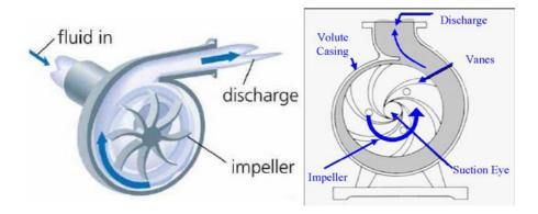
Figure 18. Centrifugal pump.
