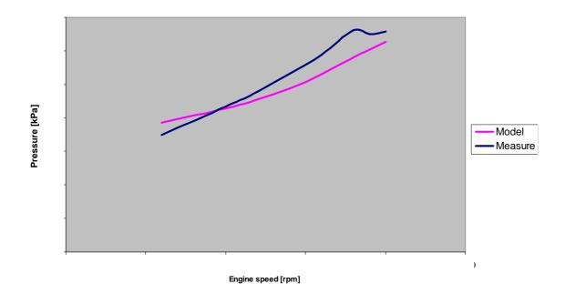
Figure 63. Pressure after transmission, Test 11.
