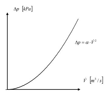
Figure 3. The system curve.
