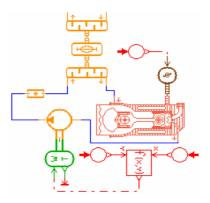
Figure 30. AMESim model of air compressor.
