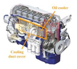
Figure 35. Oil cooling position.
