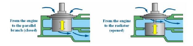
Figure 23. Closed and fully open thermostat.
