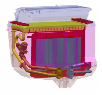
Figure 26. The cab heating system.
