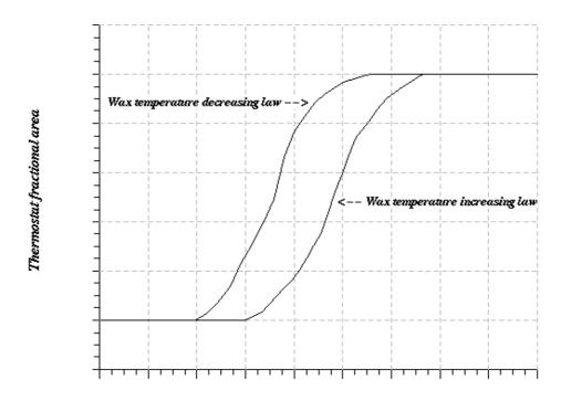
Figure 22. Characteristics curves for the thermostat.
