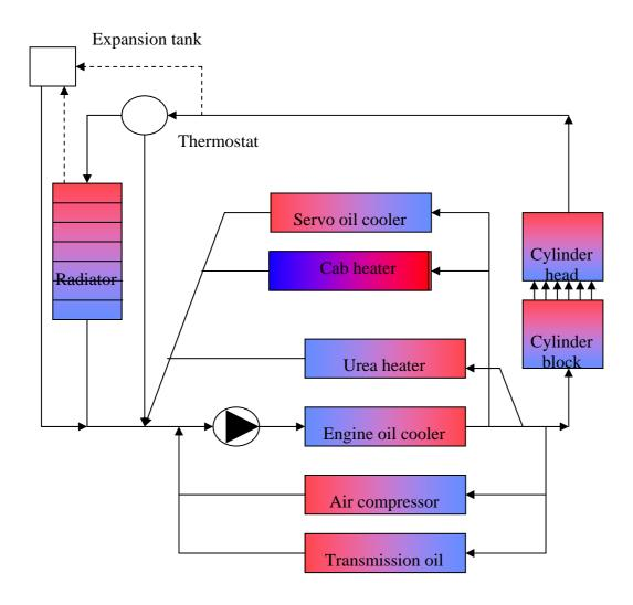
Figure 2. The cooling system.
