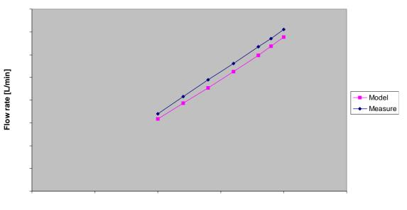
Figure 57. Flow through air compressor cooler, Test 11.
