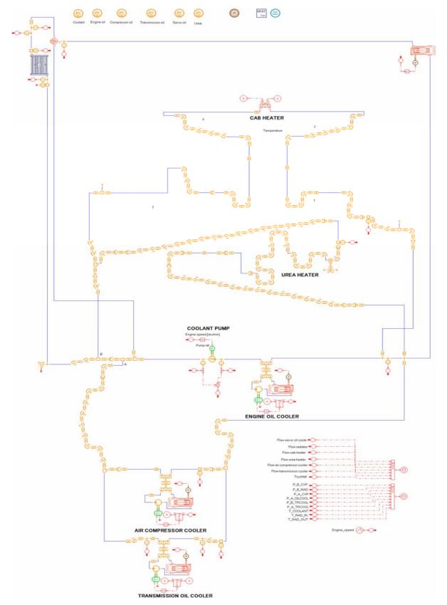
Figure 90. The AMESim model of test 11.
