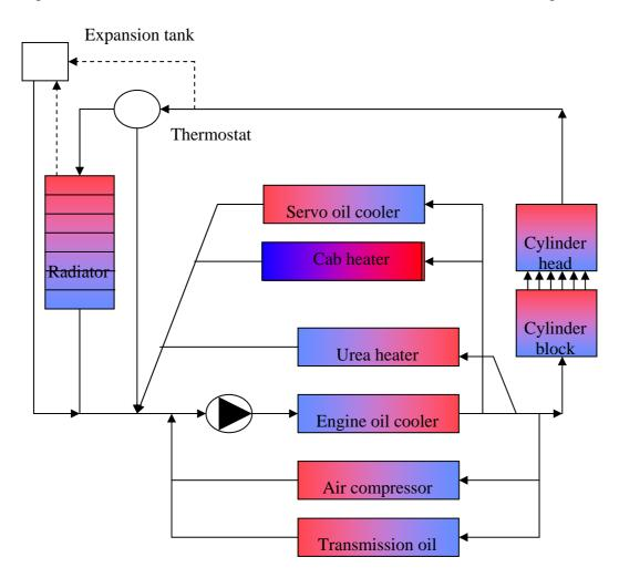
Figure 17. The coolant circuit.
