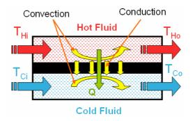
Figure 11. A general heat exchanger.
