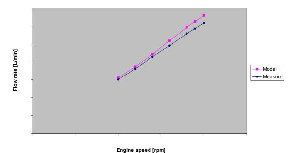
Figure 56. Flow through transmission oil cooler, Test 11.
