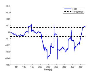
Figure 9.6. Simulation of residual generator (9.5) with a bias fault in sensor  $w_{cmp}$ .
