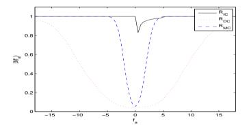
Figure 7.4. Power functions for  $R_{IC}$ ,  $R_{DC}$  and  $R_{MC}$  with actuator bias fault.
