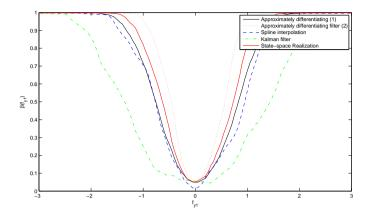
**Figure 8.4.** Power functions for residual generator  $R_2$  with various bias-errors on sensor  $y_1$ .
