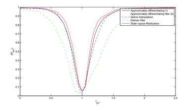
**Figure 8.5.** Power functions for residual generator  $R_2$  with various gain-errors on sensor  $y_1$ .
