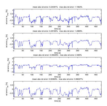
**Figure 9.2.** Validation of modified engine model. Relative error for  $w_{cmp}$  (top),  $p_{im}$  (second from top),  $p_{em}$  (second from bottom) and  $n_{trb}$  (bottom).
