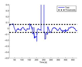
Figure 9.5. Simulation of residual generator (9.5) with a bias fault in sensor  $T_{im}$ .
