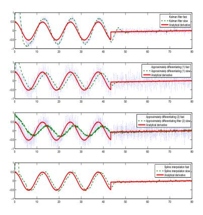
Figure 8.2. The derivative of signal estimated with three different methods.
