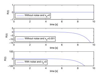
Figure 5.2. Three simulations of residual generator (5.3b) with different initial conditions.
