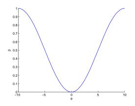
**Figure 3.2.** Typical power function  $\beta(\theta)$  for a test T(z),  $\theta = 0$  in the fault free case and  $\theta \neq 0$  when there is a fault present.
