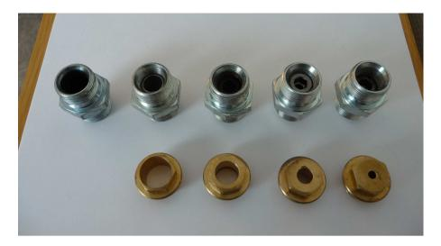
**Figure 4.2.** Bolts used to create different sizes of leakages. The upper bolts are for the EGR leakage, and have diameters from 3mm to 15mm in steps of 3mm. The lower bolts are for the boost leakages, having diameters from 5mm to 25mm in steps of 5mm. For the largest leakage on the boost-side, no bolt is used since the diameter of the bolt is as large as the desired hole diameter.
