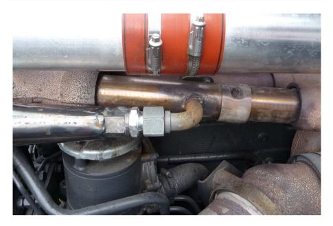
Figure 4.5. Closer view of the EGR leakage implementation. The bent pipe in the middle of the photo leads to the leakage bolt that is the splice between the two big screw nuts right after the bend.
