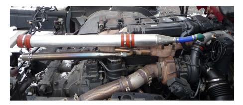
**Figure 4.3.** Overwiev of the new hardware for the leakage implementation in a truck. The upper of the two tubes in the middle of the photo is the tube for the gas from the boost-side leakage, and the lower is the tube for the gas from the exhaust-side leakage. For closeups of the holes, see Figure 4.4 for the boost-side, located to the right in the photo, and Figure 4.5 for the exhaust-side, located in the middle of the photo.
