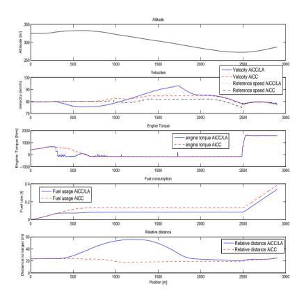
Figure 4.12. The result for Segment 3 with time gap 1 and target weight 20 tonnes.
