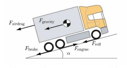
Figure 2.2. The longitudinal forces acting on a heavy vehicle.
