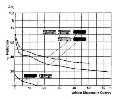
**Figure 2.3.** Reduction of  $c_D$  depending on the distance to the target, [5].
