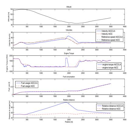
Figure 4.4. The result for Segment 1 with time gap 3 and target weight 50 tonnes.
