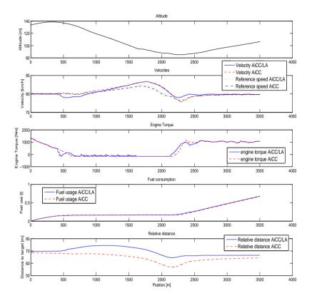
Figure 4.6. The result for Segment 1 with time gap 5 and target weight 40 tonnes.
