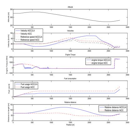
Figure 4.16. The result for Segment 3 with time gap 5 and target weight 40 tonnes.
