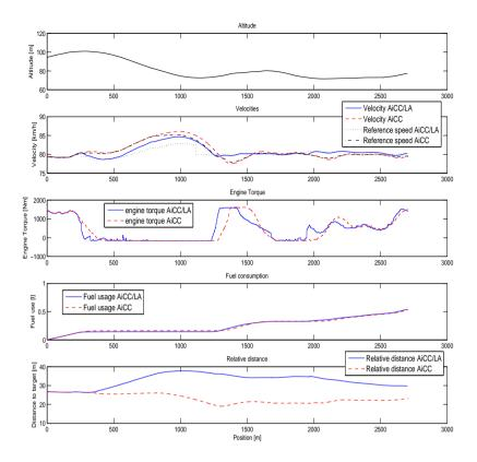
Figure 4.10. The result for Segment 2 with time gap 1 and target weight 50 tonnes.
