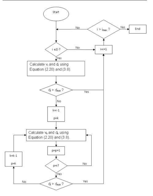
Figure 3.2. Flow chart over the process.
