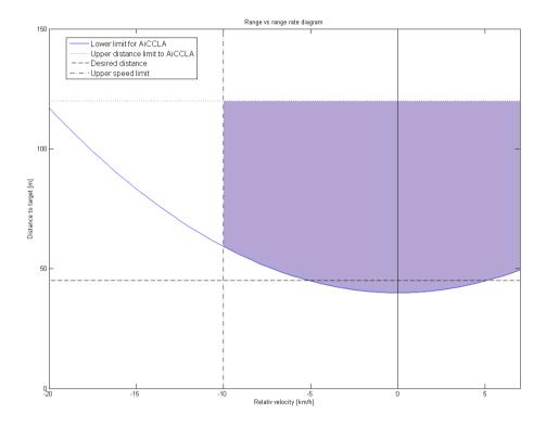
Figure 3.3. Range vs. range-rate diagram for time gap 2 seconds and target speed 80 km/h.
