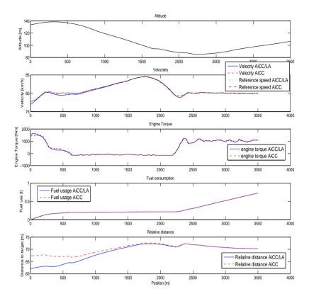
Figure 4.7. The result for Segment 1 with time gap 5 and target weight 50 tonnes.
