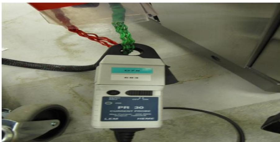
Figure 3.5: Current Probe Model PR30
