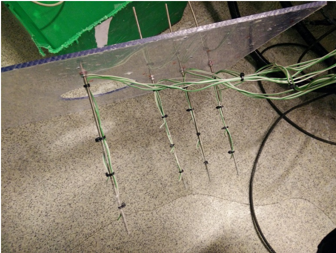
Figure 4.4: Sensor plate with mounted sensors
