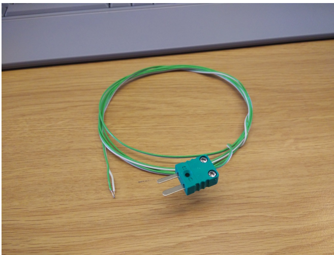
Figure 4.12: The thermocouples used for measuring temperature
