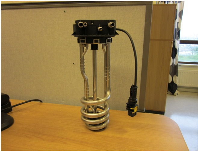
Figure 4.5: The combined heating armature and AdBlue pickup
