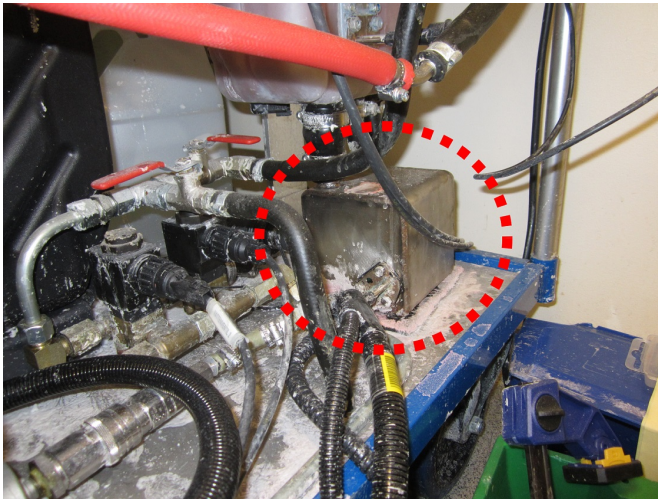
Figure 4.7: The coolant heater
