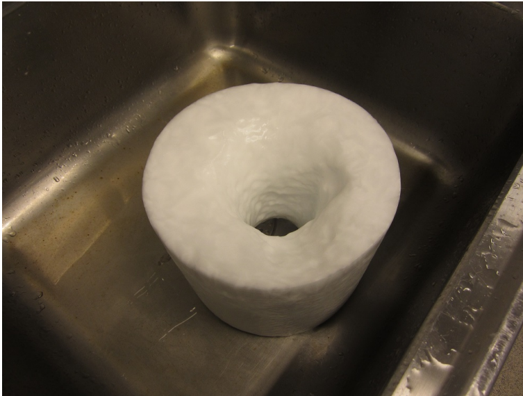
Figure 2.1: A sample of frozen AdBlue
