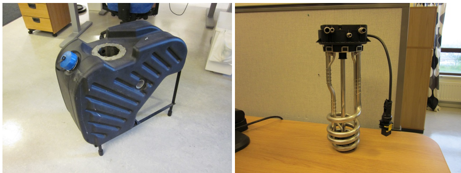
Figure 1.2: Euro 5 AdBlue tank and combined heat spiral and urea delivery unit
