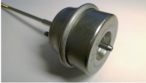
Figure 2.4: Pneumatic actuator for wastegate valve with control rod to the left and vacuum-feeding nozzle to the right.
