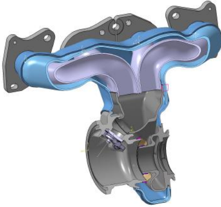
Figure 2.1: 3D model of the exhaust manifold. Shows how the exhaust manifold is built of multiple layers.
