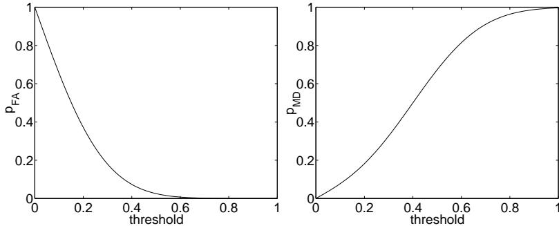
FIGURE 2: Probabilities of FA and MD as functions of threshold size. for a test.
