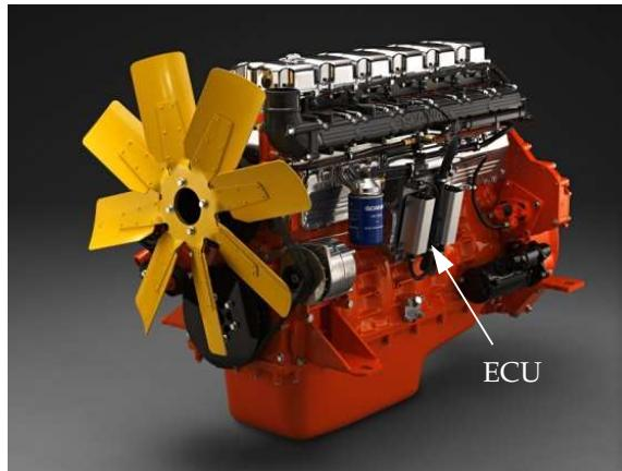
FIGURE 1.2: The figure shows a 12 liter industrial engine from Scania ([Scania, 2007](#)). The engine ECU is attached to the side of the engine and its objective is to supervise the engine for abnormal behavior and to control the engine such that emissions are minimized and performance maximized.
