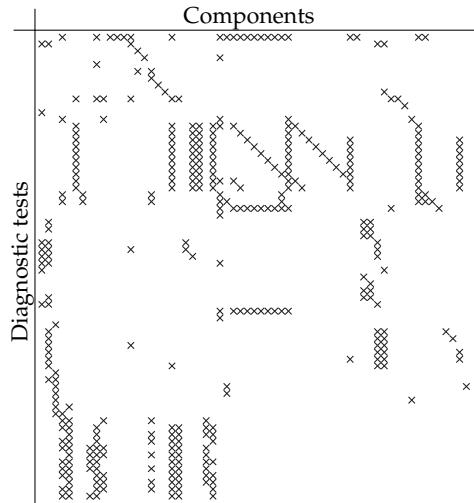
FIGURE 2.1: The isolation structure in the engine management system, which controls and supervises the engine in a Scania heavy duty truck.
