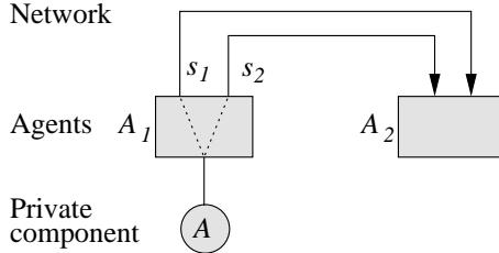
FIGURE 10: An example of a system consisting of two agents, one component, and two signals.
