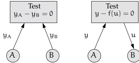
FIGURE 2.4: The figure shows two different tests that supervise components. The left test is described in Example 5 and the right is described in Example 6.
