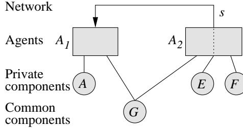
FIGURE 2: An example of a system consisting of two agents, four components  $A$ ,  $E$ ,  $F$ , and  $G$ , and one signal  $s$ . The agents use the components connected with lines.
