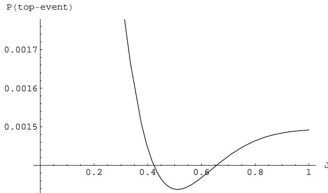
FIGURE 10: Probability for the top event as function of the threshold.
