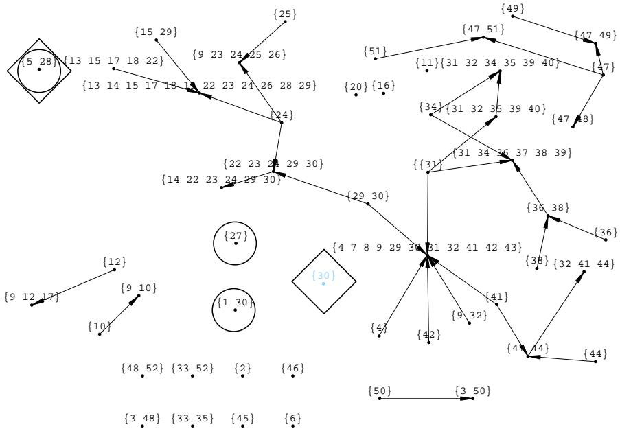
FIGURE 11: The updated DAG G for the SCR with conflicts displayed at the corresponding vertex. Diagnostic tests that have been evaluated after they were considered meaningful for the suspected components are marked with a diamond.
