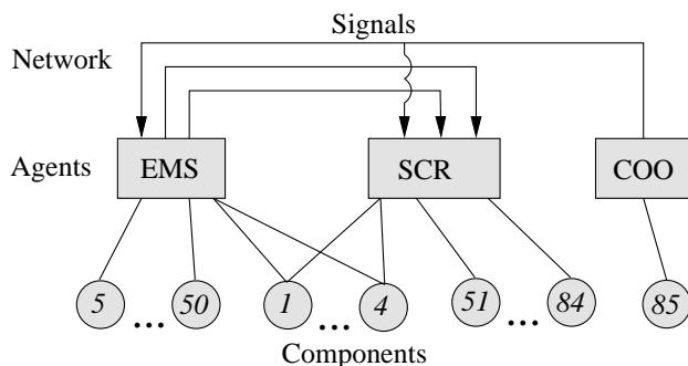
FIGURE 2.3: A schematic overview of the distributed system used in the Scania application.
