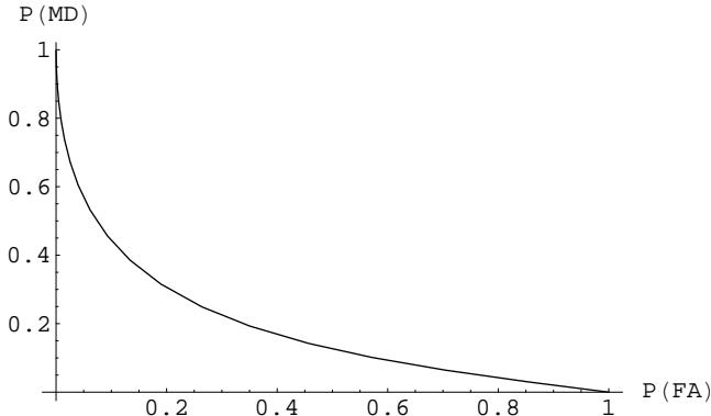
FIGURE 8: The curve indicates performance of a diagnosis algorithm in a  $P_{FA}/P_{MD}$  diagram.
