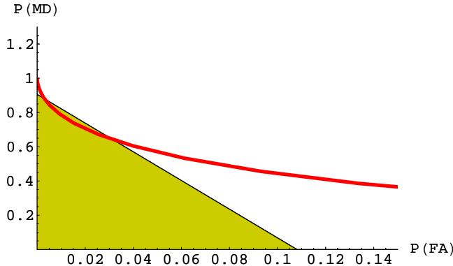
FIGURE 9: Feasible diagnosis performance (shaded) and performance of the detection algorithm (curve).
