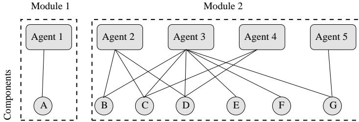
FIGURE 3: The agents have calculated sets of minimal local diagnoses that includes the components connected with lines. The agents have been partitioned into two modules.
