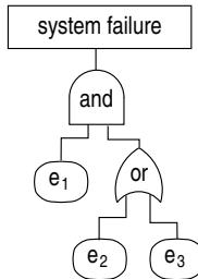
FIGURE 1: A fault tree for the system in Example 1.
