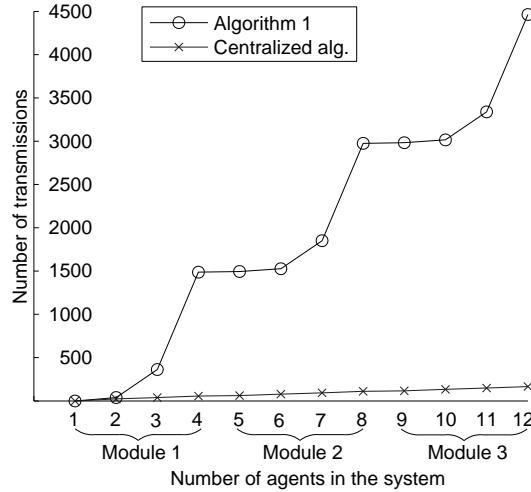
FIGURE 5: Number of transmissions on the network.
