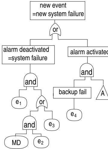
FIGURE 7: A simplification of the fault tree in Figure 3.
