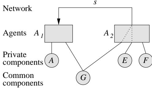
FIGURE 11: An example of a two agent system where the signal depends on a common component.
