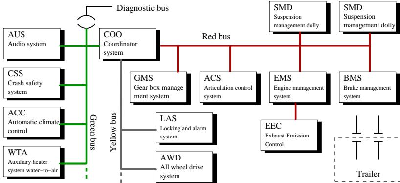
FIGURE 1: A part of the distributed system in Scania vehicles.
