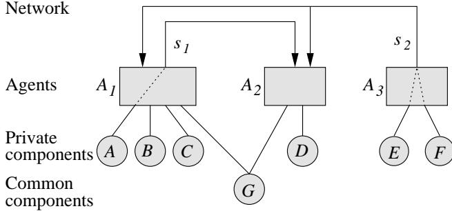
FIGURE 3: An example of a system consisting of three agents, seven components, and two signals. The components connected with lines are used by the corresponding agents.
