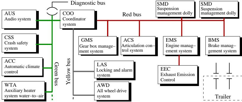
FIGURE 1: The distributed system in current Scania vehicles.
