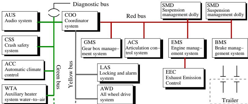
FIGURE 1.4: The distributed system in current Scania heavy-duty vehicles. The distributed system consists of dozens of ECUs, such as the CSS crash safety system that is responsible for protecting the driver and the passengers in case of a road traffic accident.
