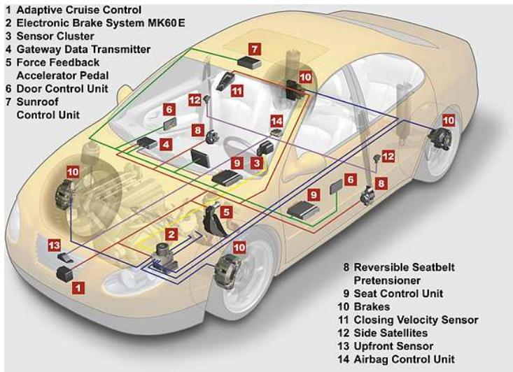
FIGURE 1.5: The distributed system in a personal automotive vehicle (AA1CAR, 2007). Multiple ECUs are distributed over the vehicle and are responsible for control and supervision of different parts of the vehicle, such as the adaptive cruise control or the airbag control unit.
