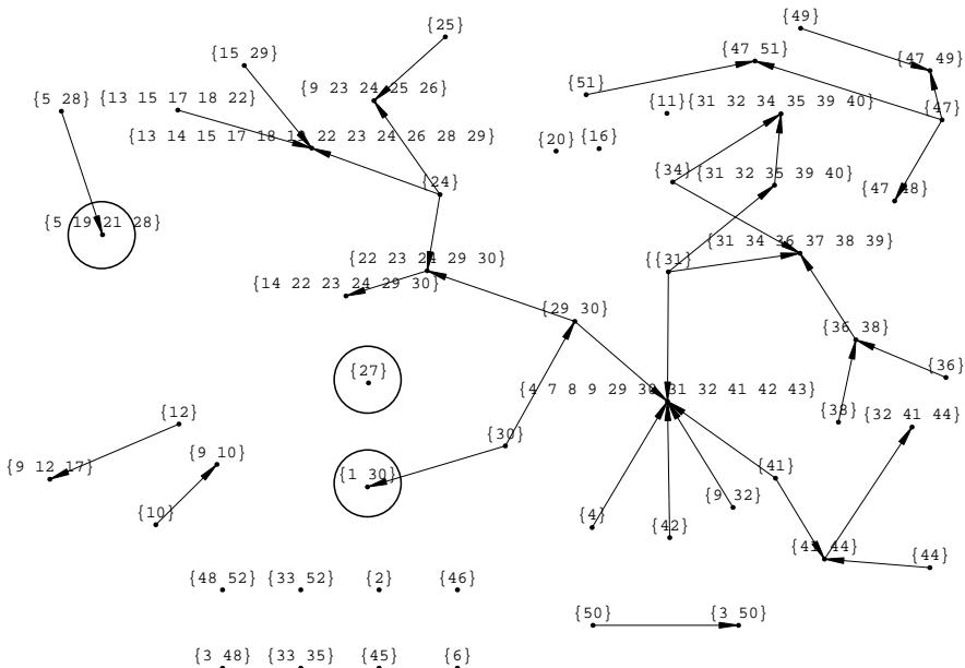
FIGURE 6: The updated DAG for the SCR with marked vertices circled.
