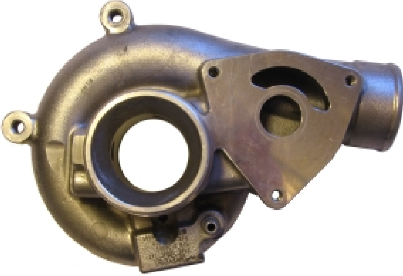
Figure 2.2: Compressor scroll with built in recirculation valve or surge valve. For surge control, air is recirculated from the outlet duct through the banana shaped hole at the upper right, through the circular hole close to the banana, and then through internal channels to the compressor inlet which is at the center of the scroll. Control of the surge valve is discussed in Paper 1, and this particular scroll belongs to one of the turbos ran in surge for the measurements of Papers 1 and 4.
