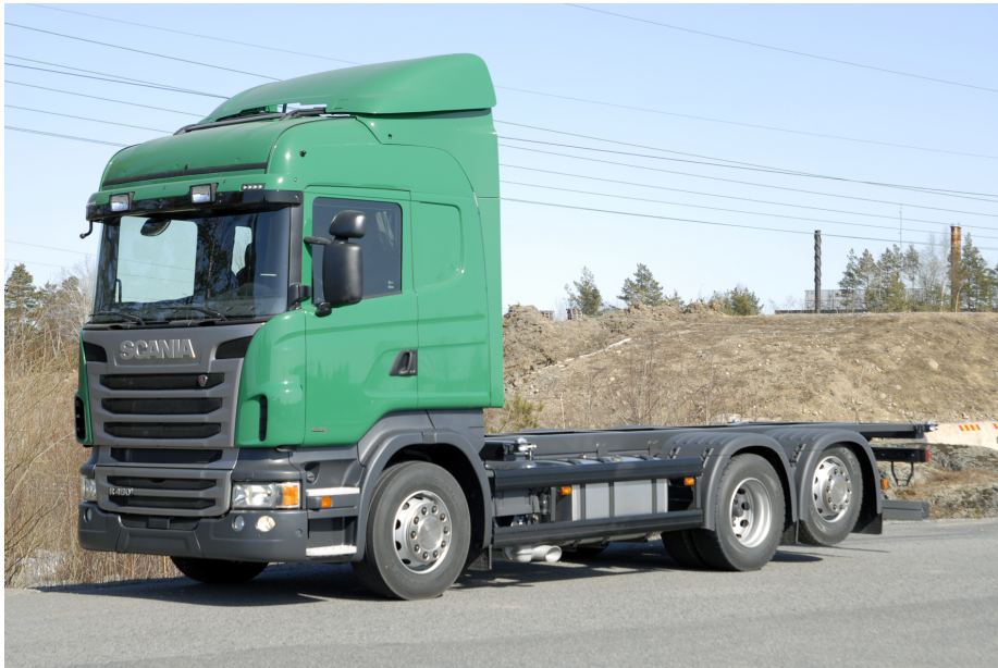
Figure 1: A photograph of the test vehicle Fronda. It is unloaded in the picture but during the experiments it has been loaded to total weight of 21 metric tonnes.
