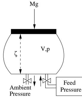
Figure 1: Principle sketch of the bellows.
